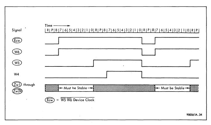
Figure 3-4. TMCC Input Timing, Synchronous Clock
