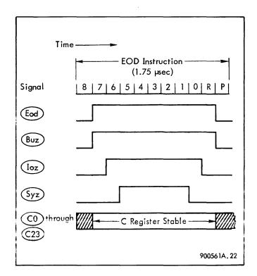
Figure 2-2. Signals Generated by EOD Instruction
