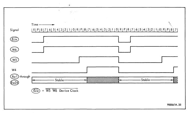
Figure 3-5. TMCC Output Timing, Synchronous Clock
