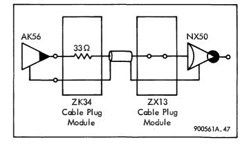
Figure 4-7. High-Speed Output, Circuit Type O3
