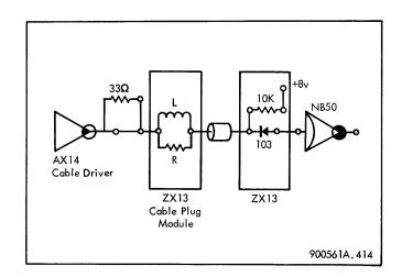
Figure 4-14. AX14 Driving Low-Speed Input
