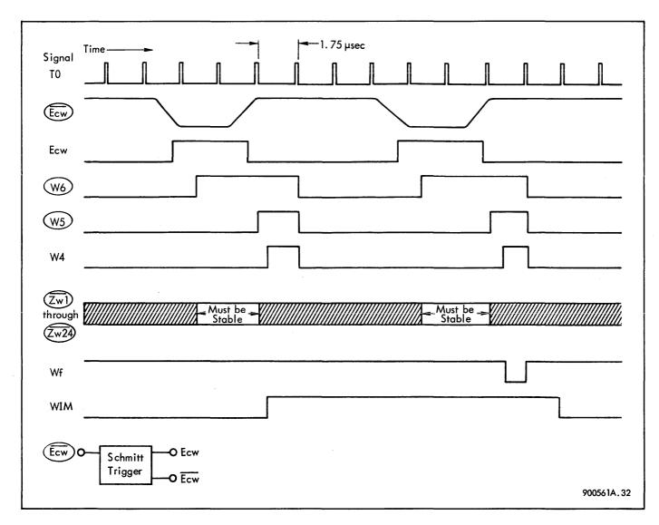
Figure 3-2. Input Timing Characteristics Asynchronous Mode
