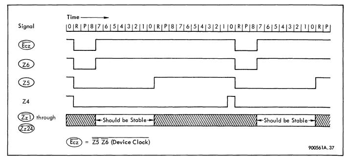
Figure 3-7. DACC Timing, Synchronous Input Mode
