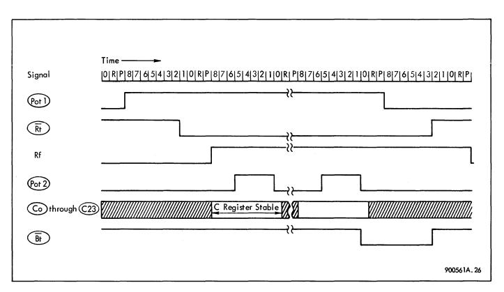
Figure 2–6. Signals Generated by 925 BPO Instruction
