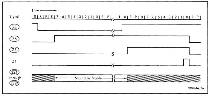
Figure 3-6. DACC Timing, Asynchronous Input Mode
