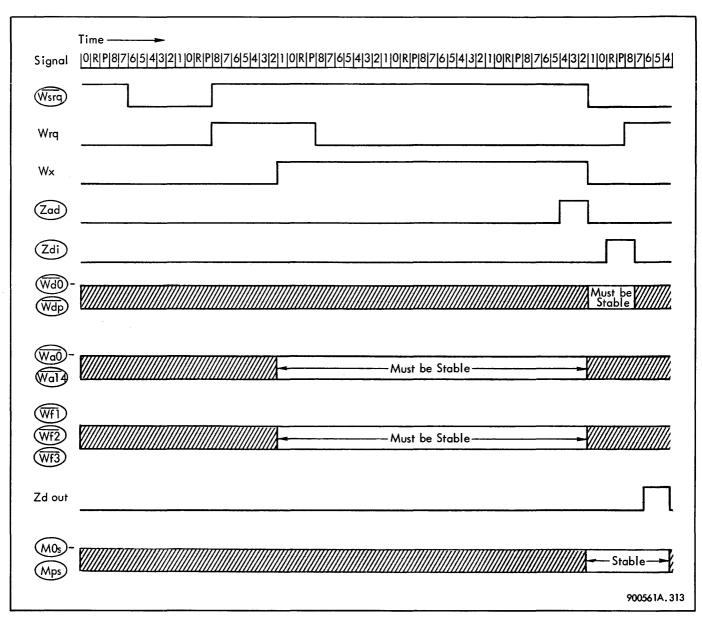
Figure 3-13. Timing Diagram DSC-II Input/Output Using Internal Interlace
