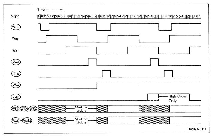
Figure 3-14. Timing Diagram DSC-II Word Increment Function
