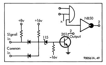
Figure 4-9. Interface Inverter, NB50
