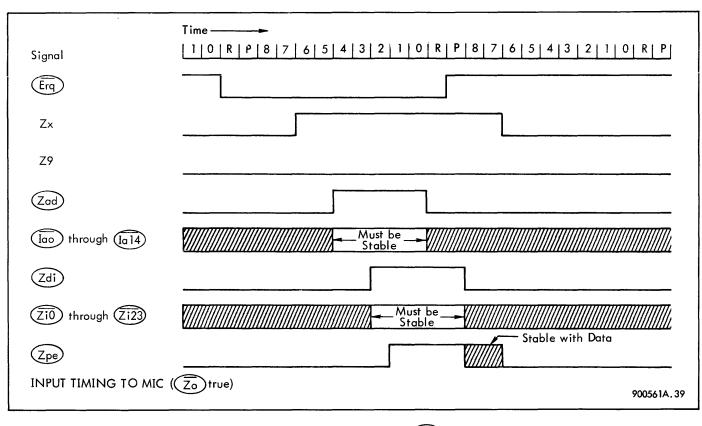
Figure 3-9. MIC Input Timing ( Zo True)
