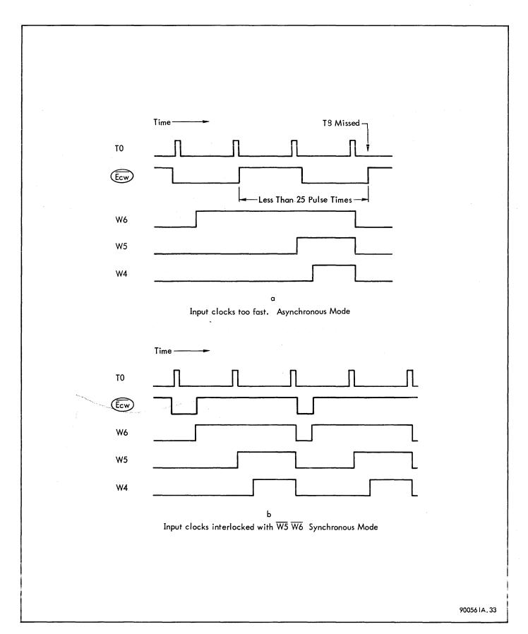
Figure 3-3. Input Clock Timing Diagram
