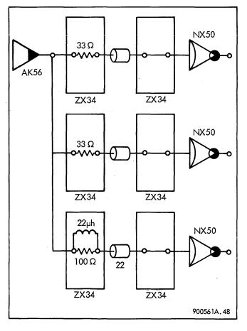
Figure 4-8. Cable Driver AK56 Loading
