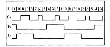
The Cz pulse is a clock generated in the DMC for use by the DSC's. Tx and Ty timing pulses are made available for use by external devices. The computer timing pulses are not available to the DSC's or to the external devices.
