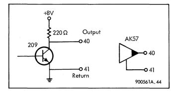
Figure 4-4. Cable Driver AK57 Output
