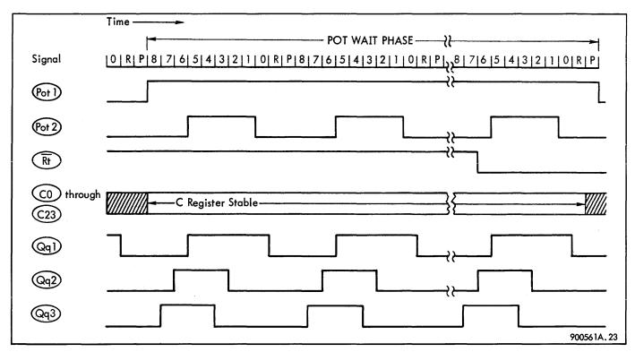
Figure 2–3. Signals Generated by POT Instruction
