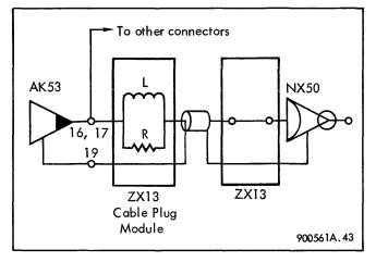
Figure 4-3. Typical Interface Connection, Low-Speed Outputs, Type O1
