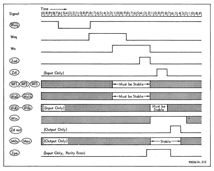
Figure 3-12. Timing Diagram DSC-II Terminating Input/Output with External Address
