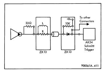
Figure 4-11. Input Circuit Type I3
