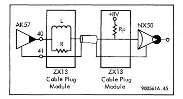
Figure 4-5. Low-Speed Output, Circuit Type O2
