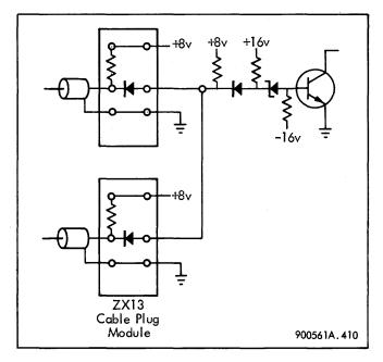
Figure 4–10. Input Signal Gating
