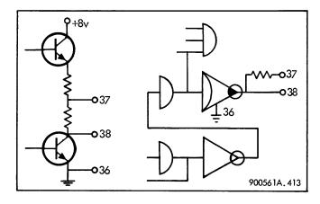
Figure 4-13. Low-Speed Input Cable Driver AX14
