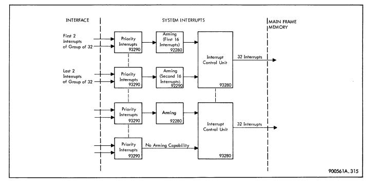
Figure 3-15. System Priority Interrupt Configuration
