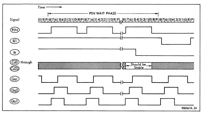
Figure 2-4. Signals Generated by PIN Instruction
