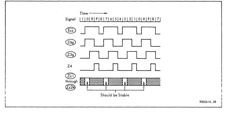
Figure 3-8. DACC Timing, High-Speed Synchronous Input Mode
