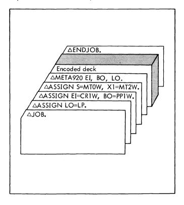
Assemble META-SYMBOL symbolic and encoded input from card reader. (Note that  $\triangle$  EOF indicates termination of SI.)
