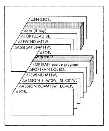
Compile and execute a FORTRAN program input from paper tape. If the source tape does not end with a  $\triangle EOF$ , control must be transferred to MONARCH manually.
