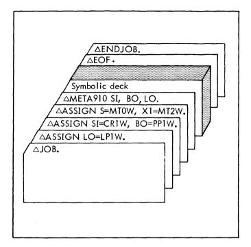
Assemble a META-SYMBOL encoded deck to produce an object program for 920/930. (Note that encoded deck requires no EOF indication.)
