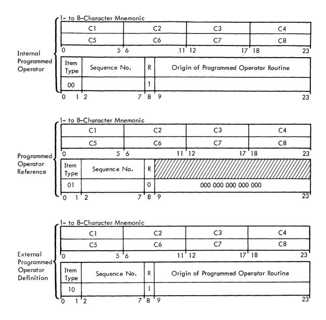
R = 1 iff origin of Programmed Operator Routine is relocatable. The sequence number indicates the order in which the definitions or references occurred in the source program.
