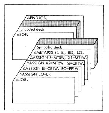
Assemble META-SYMBOL encoded deck with symbolic corrections on a 900 Series Computer to produce an object program to run on 9300.
