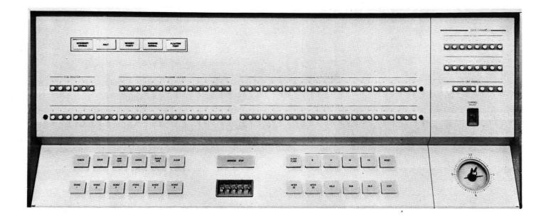
Figure 5-1. SDS 9300 Control Panel
