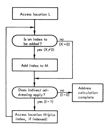
Figure 1-3. Address Calculation
