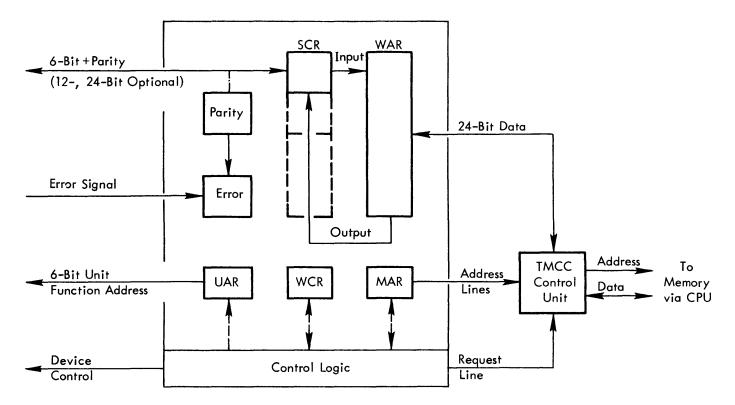
Figure 4-1. Typical SDS 9300 Time-Multiplexed Communication Channel, Block Diagram
