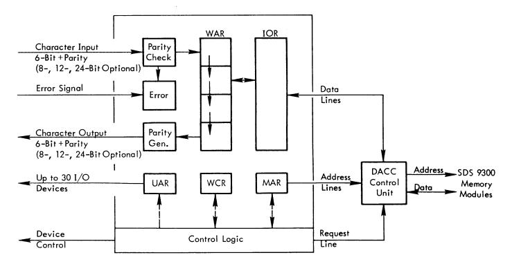
Figure 4-2. Typical SDS 9300 Direct Access Communication Channel, Block Diagram
