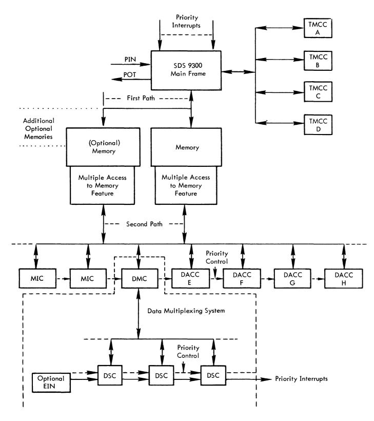
Figure B-1. SDS 9300 Overall Computer Configuration
