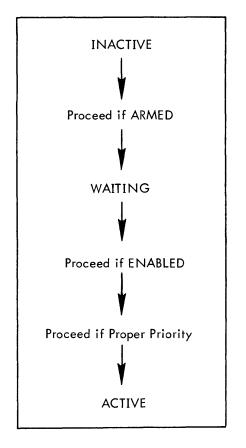
Figure 3-1. Interrupt Arm/Enable Response
