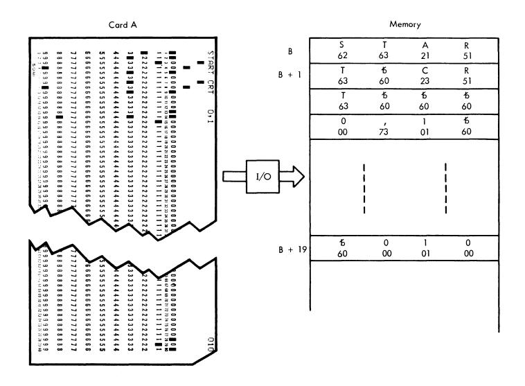
Figure 6-1. Card Read Into Memory in Hollerith
