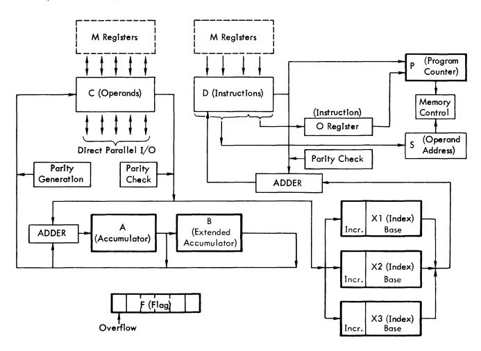
Figure 1-2. Basic Register Flow Diagram
