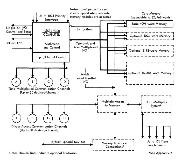
Figure 1-1. SDS 9300 Computer Configuration
