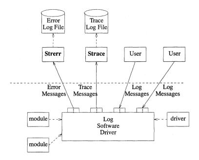
Figure 6-5 Error and Trace Logging
