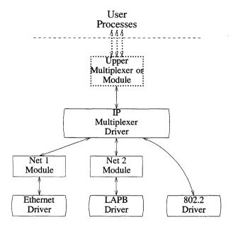
Figure 6-3 Internet Multiplexing Stream
