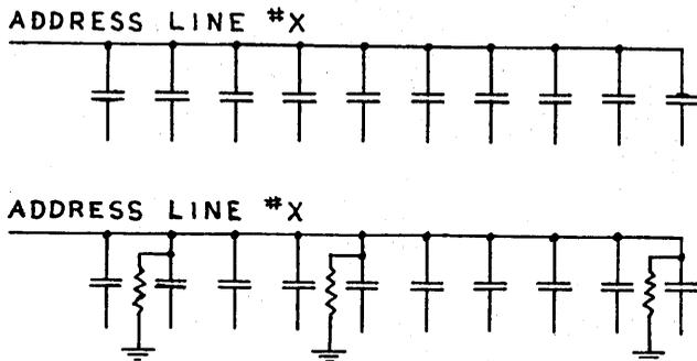
REMEMBER, SUCH DEFECTIVE DEVICES MAY WELL PASS AN OPERATIONAL TEST IN A TEST SET UP WHEN THEY ARE THE ONLY DEVICE BEING DRIVEN. WHAT IS AN EASY WAY FOR THE READER TO CHECK FOR THIS TYPE OF DEFECT? A VERY CRUDE TEST, BUT ONE THAT WORKS QUITE SATISFACTORILY CAN BE MADE WITH A SIMPLE OHM METER!
