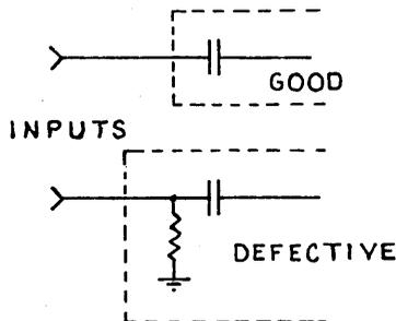
A MEMORY ELEMENT THAT HAS A "GOOD" (ESSENTIALLY CAPACITIVE) INPUT WILL REQUIRE VERY LITTLE DRIVING POWER FROM THE CIRCUIT THAT ACTIVATES THE INPUT - BE IT AN ADDRESS OR DATA LINE. WHEN THE INPUT LEVEL CHANGES, THE DRIVING CIRCUIT ONLY HAS TO "SOURCE" OR "SINK" ENOUGH CURRENT TO CHARGE OR DISCHARGE THE INPUT CAPACITANCE PLUS A VERY SMALL AMOUNT OF SO CALLED "LEAKAGE" CURRENT (IN THE ORDER OF NANO-AMPERES, OR MILLIONTHS OF AN AMPERE).
