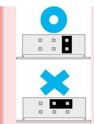
Only one jumper should be installed on the jumper connector. If more than one jumper is installed, the drive may malfunction or be damaged.
