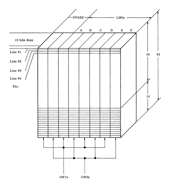
Figure 3-1. Schematic Appearance of CCM Memory Layout
