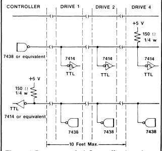
Figure 4. Recommended Controller Interface Circuit.
