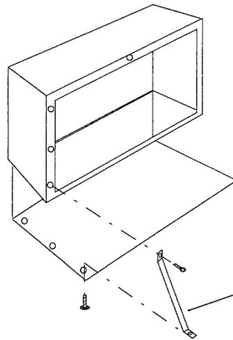
Installing the support bracket as shown will allow you to place the tape drive sideways as shown.
