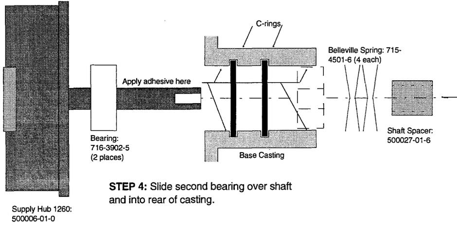
**STEP 4:** Slide second bearing over shaft and into rear of casting.
