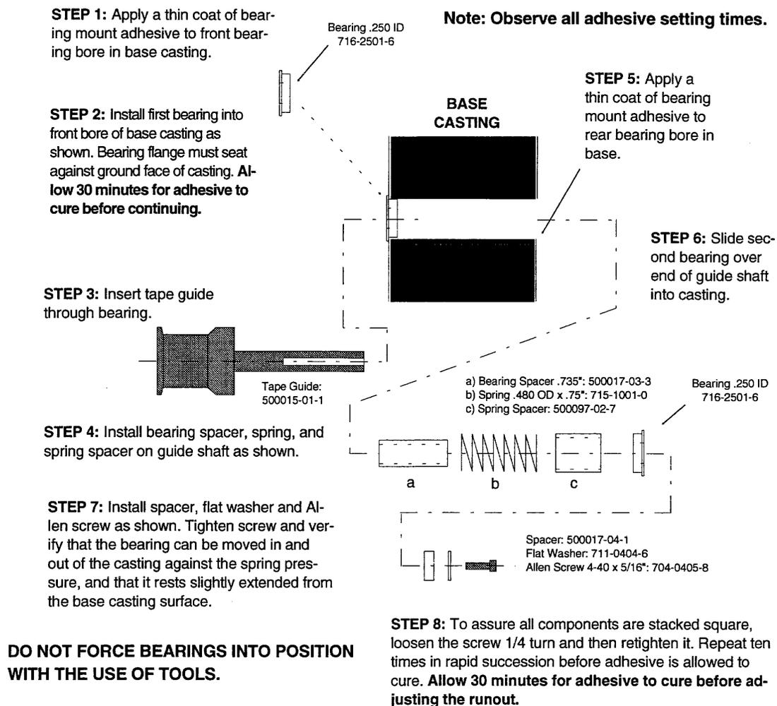
Figure 8-3 Fixed Tape Guide Assembly
