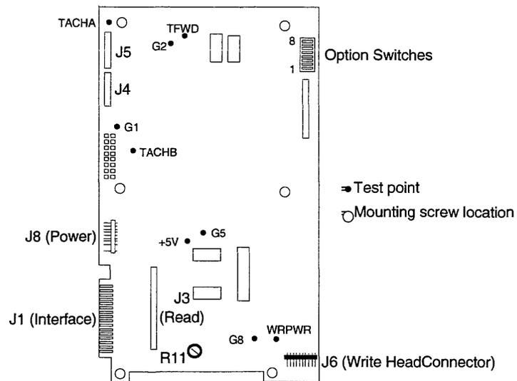
**Figure 6-3** Write/Controller Layout
