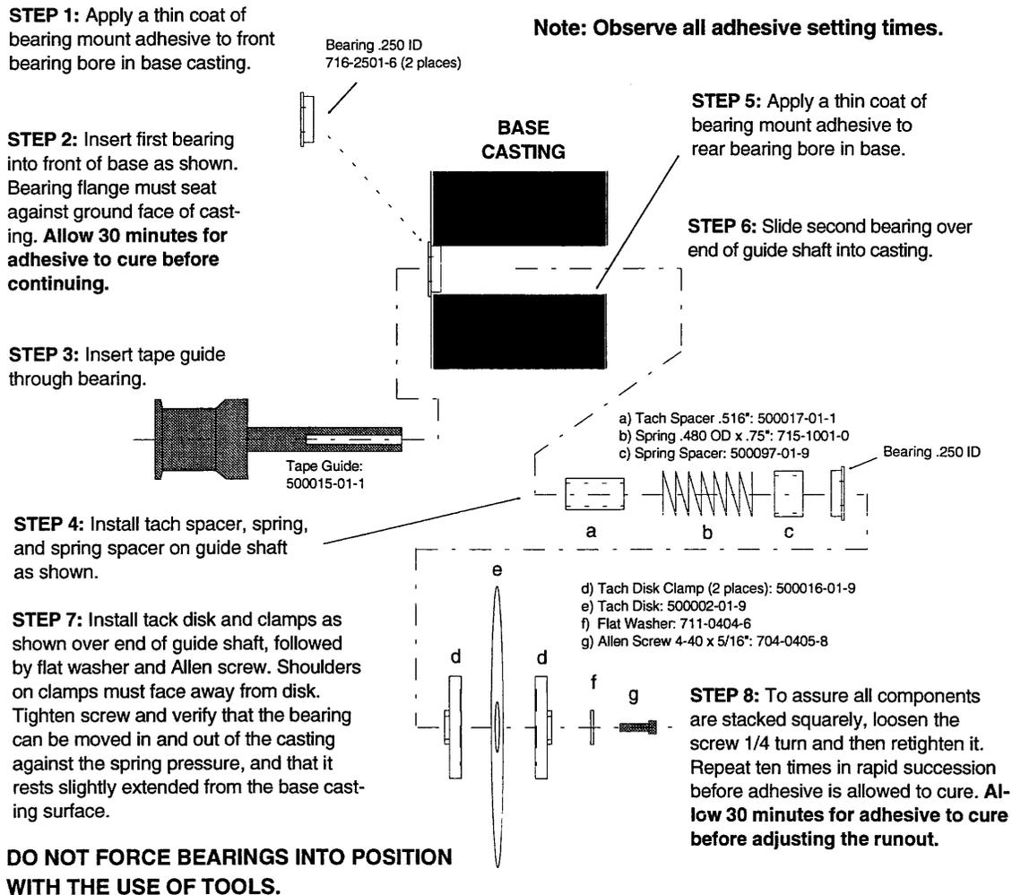
Figure 8-2 Tachometer Tape Guide Assembly
