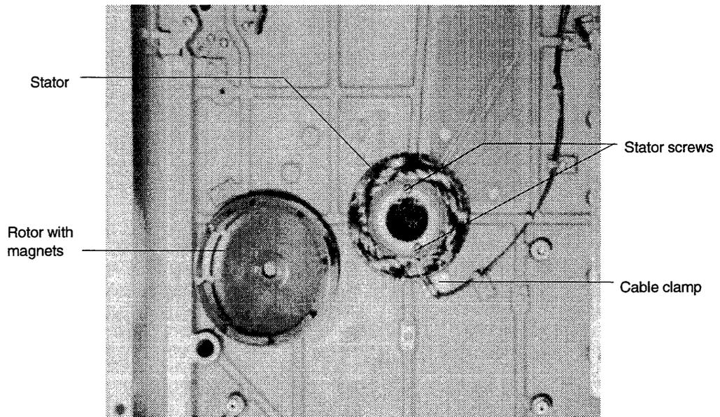
Figure 6-5 Motor Rotor and Stator
