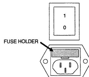
Figure 6-2 AC Plug and Fuse Holder
