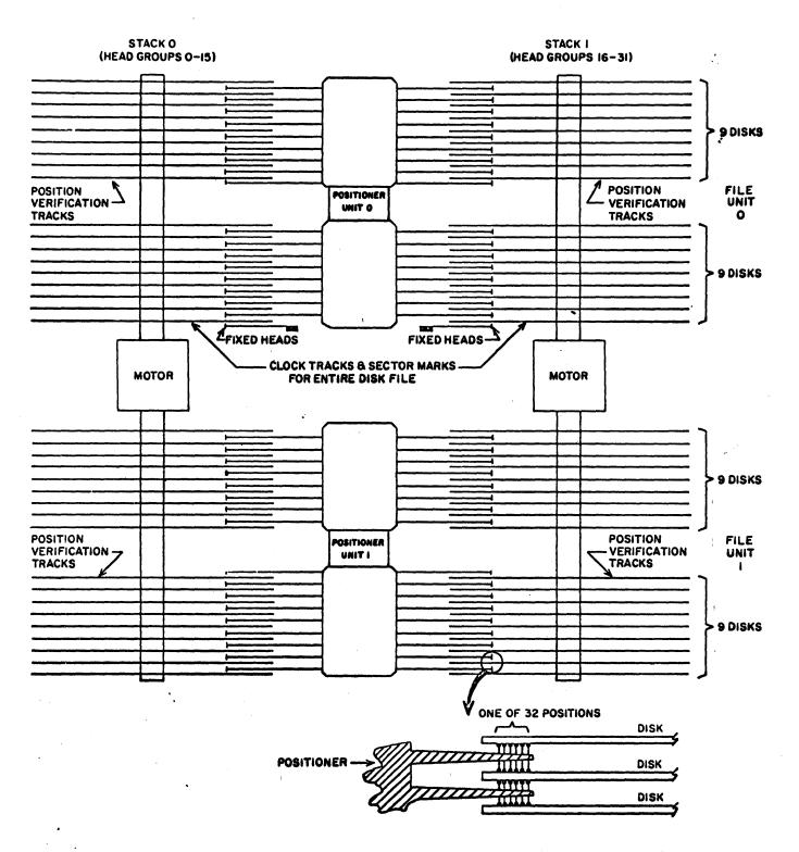
Figure 5. 808 Disk File Disks and Positioners
