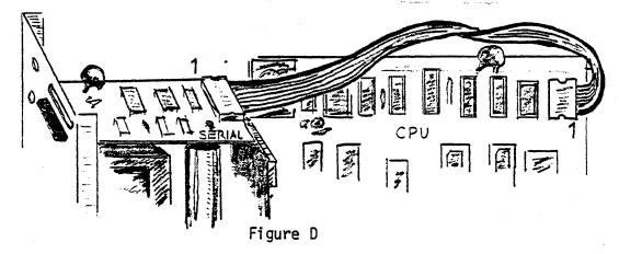
Note that there are two output port connectors on the upper right corner of the processor board, connected in parallel. The serial option can be plugged into either port. Pre-bend the ribbon cable to clear the small components on the end of the board.
