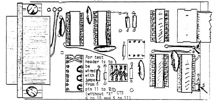
Before mounting the serial option card on the back panel, check to see that it is operating correctly. Attach the ribbon cable from the mini-card to the processor board, making sure that pin 1 is down.
