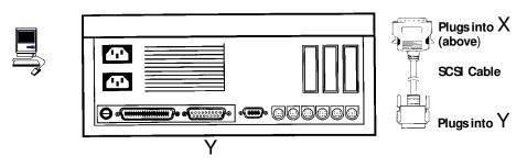
If you are installing more than one UltraPleX external drive (or one external UltraPleX and other external SCSI peripherals), connect them as shown below:
