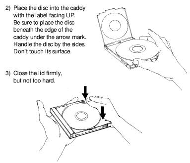
Caution: If the caddy appears defective (e.g., warped, cracked, or bent) do not insert it into the drive. A defective caddy can become stuck inside the drive, requiring the drive's return to Plextor for service. If your caddy appears defective, promptly replace it with a new one.
