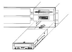
You now need to make the power connection. In most computers you will find additional power connectors that are ready for use. Check the cable running from your power supply to your hard disk and see if it has extra connectors on it. If so, you can plug one of these into the power connector found on the rear panel of the CD-ROM drive.
