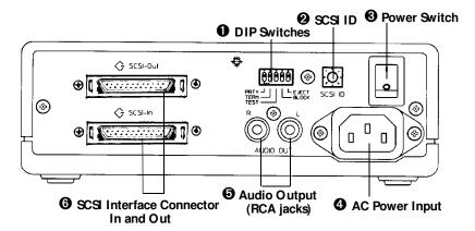
**1 DIP Switches:** Use to set parity, term, test, block size, and eject lock options. Leave these switches at their factory settings unless one of the following pertain to you:
