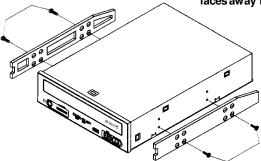
There are four holes provided on each side of the drive. To mount an internal drive in most computers, the rails should be fastened to the lower pair of holes. In some instances you may need to fasten the rails to the upper set of holes.
