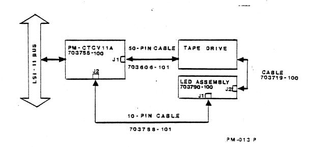
Figure 2-2. PM-CTCV11A Cabling
