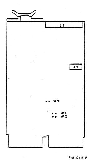
Figure 2-1. PM-CTCV11A Jumper and Connector Locations
