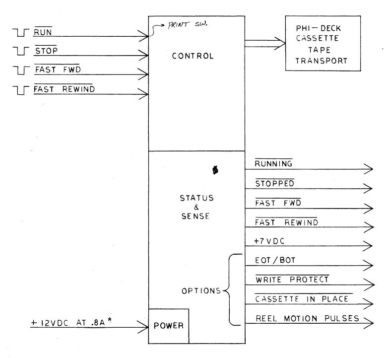
All non-optional input and output lines are DTL - TTL and CMOS compatible. Option lines are either DTL - TTL compatible logic signals or analogue signals. Discrete speeds available are 1-7/8, 2, 3-3/4, 4, 5, or 6 IPS.
