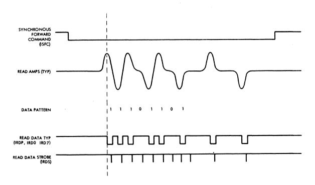
Figure 5. Typical Read Timing Diagram
