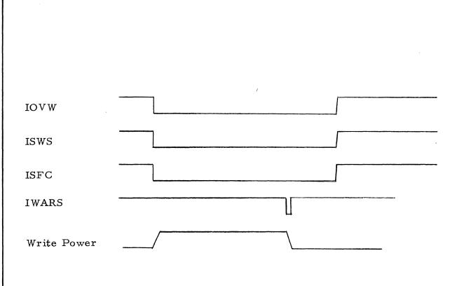
Figure 7. Overwrite Timing Diagram
