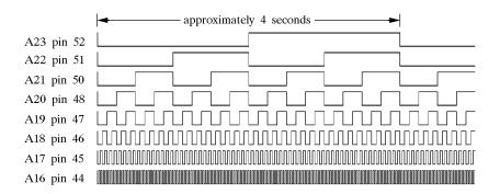
Fig. 7-4. Address bus waveforms during testing.
