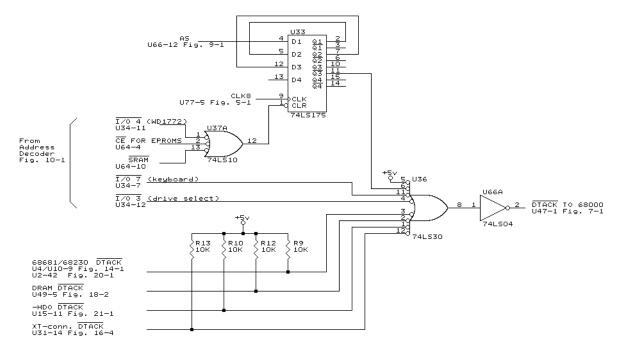
Fig. 11-1. DTACK generator circuit.
