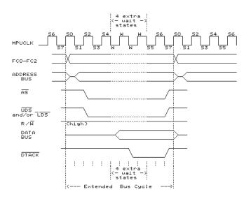
Fig. 6-3. Extended read cycle timing.
