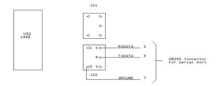
Fig. 14-2. Serial connector wiring.
