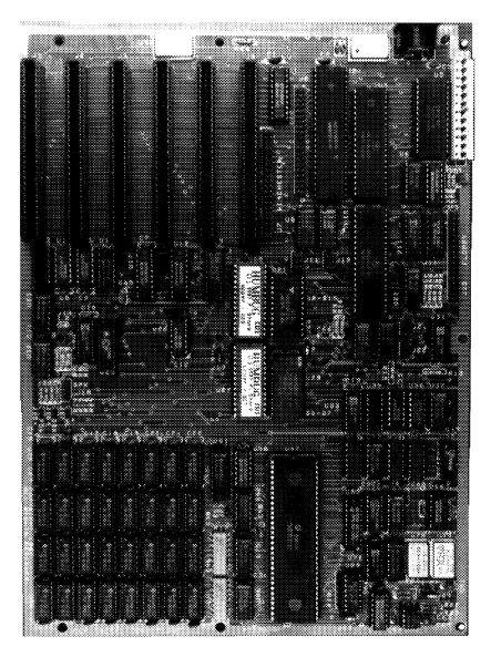
Fig. 1-1. The SK68K Printed Circuit Board.
