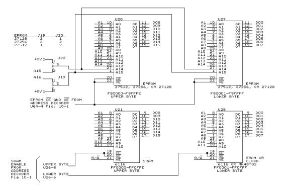
Fig. 12-1. EPROM and static RAM wiring.
