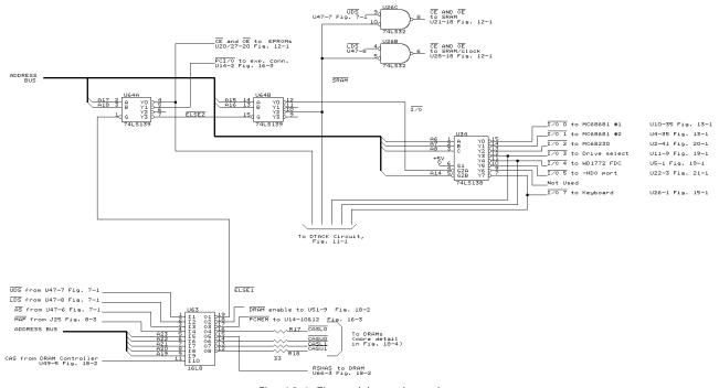
Fig. 10-1. The address decoder.
