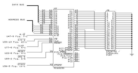
Fig. 20-1. Printer / parallel port.
