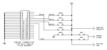
Fig. 19-2. Drive select circuitry in a typical drive.
