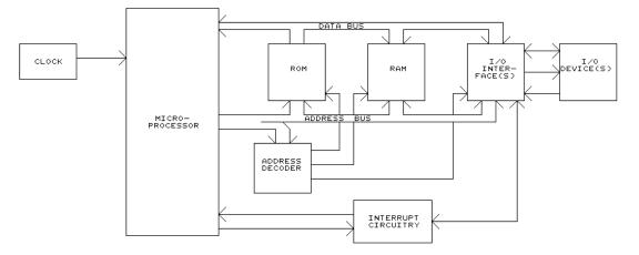
Fig. 1-2. Typical computer block diagram.
