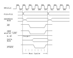
Fig. 6-2. Normal read cycle timing
