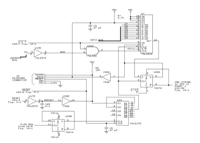
Fig. 15-1. PC-compatible keyboard interface.
