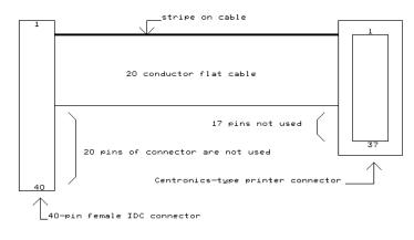
Fig. 20-2. Parallel printer cable.
