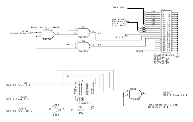
Fig. 21-1. -HDO hard disk controller port.
