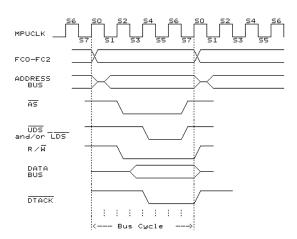
Fig. 6-4. Normal write cycle timing.
