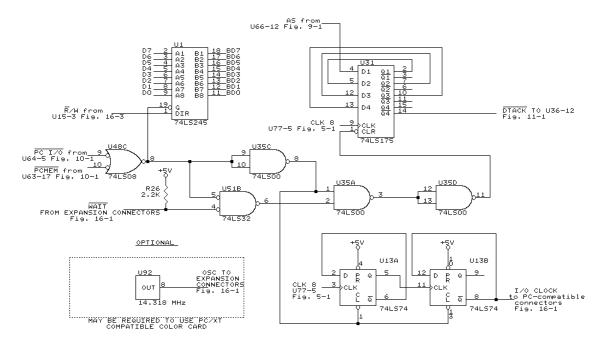
Fig. 16-4. Miscellaneous expansion circuitry.
