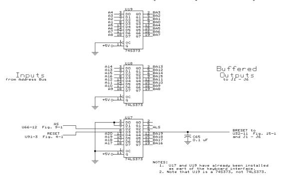
Fig. 16-2. Address bus buffers.
