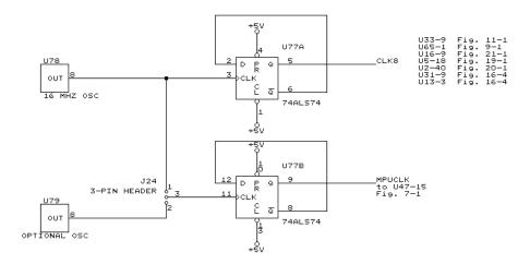
Fig. 5-1. Main clock circuit.
