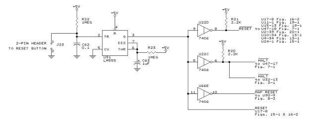
Fig. 4-1. The RESET circuit.
