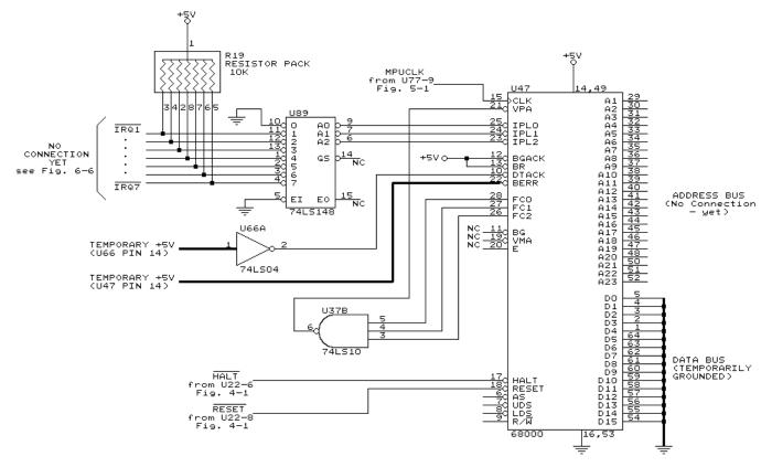
Fig. 7-1. Test circuit for the 68000.
