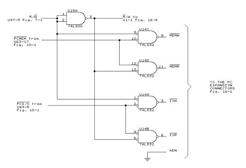
Fig. 16-3. Memory and I/O select logic.
