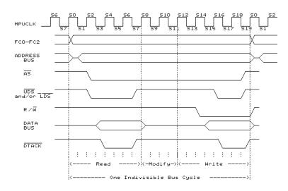
Fig. 6-5. Read-modify-write cycle timing.
