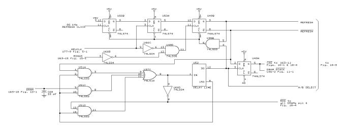
Fig. 18-2. DRAM timing circuits.
