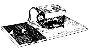
Fig. 2-2. One way to mount the board and supply.
