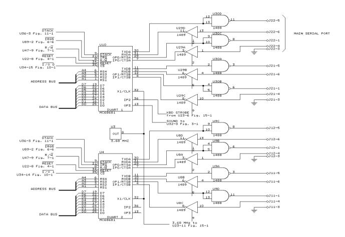
Fig. 14-1. Serial port circuitry.
