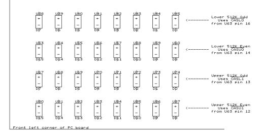
Fig. 18-5. Physical layout of the 32 RAM ICs.
