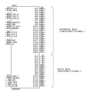
Fig. 6-1. 68000 microprocessor pinout.
