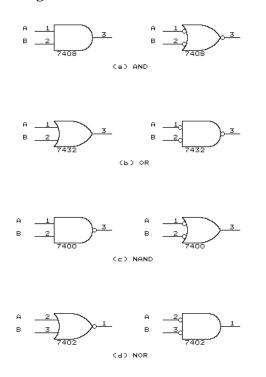
Fig. 8-2. Logic gate equivalents.
