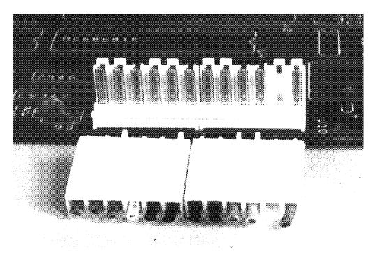
Fig 2-3. Power connectors and plugs. Note how the tabs match
