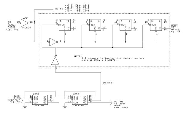
Fig. 9-1. Circuit to generate BERR.
