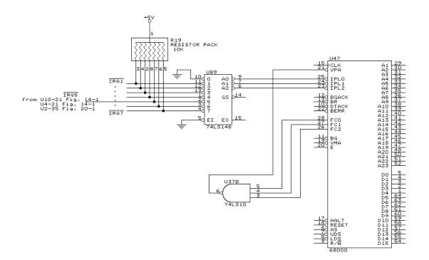
Fig. 6-6. 68000 Interrupt circuitry.
