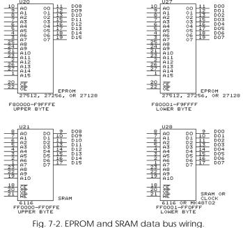
Fig. 7-2. EPROM and SRAM data bus wiring.
