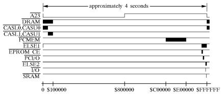
Fig. 10-2. Address decoder output waveforms.
