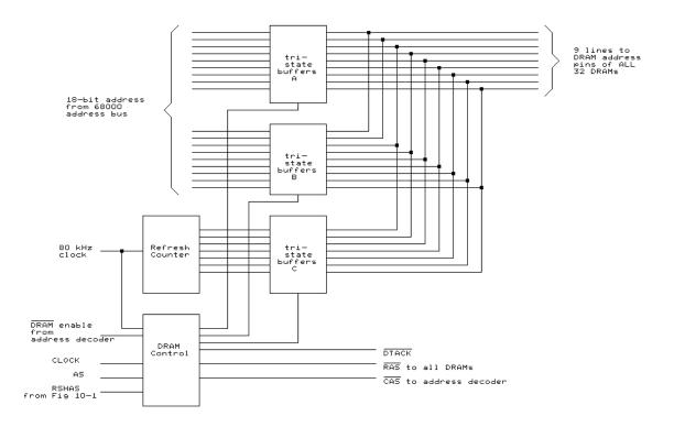
Fig. 18-1. DRAM section block diagram.
