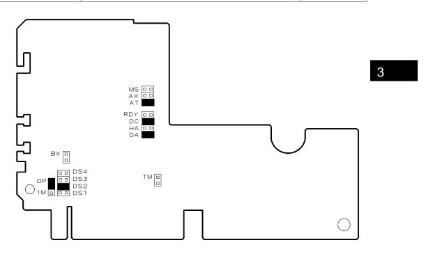
Note: Jumpers EX, GX, DD and TH have been removed from drive JU-475-5 C08 starting from this drive's level 03 (March, '94). To set the disk change mode 2 on this drive (as used on L1 with GO280D, FP1 fw2.4, FP4 fw3.7), solder a 15 Khom resistor at R18. The JU-475-5 C20 drive will no longer be available from March, 1994; instead, you can use drive JU-475-5 C08 by inserting jumper BX.
