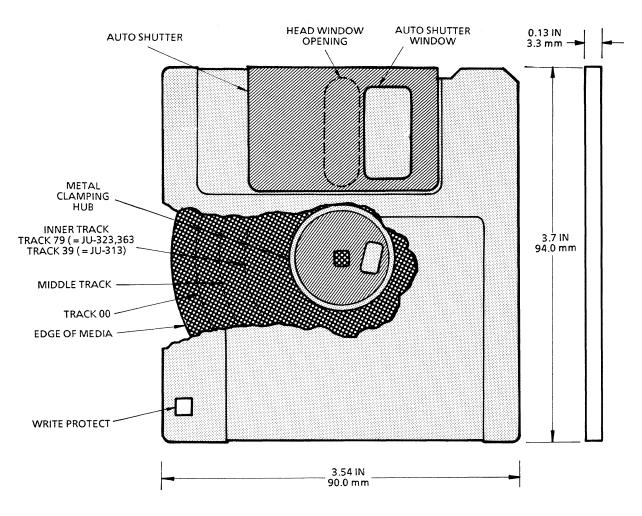
FIGURE 8-2 MICROCARTRIDGE NOMENCLATURE
