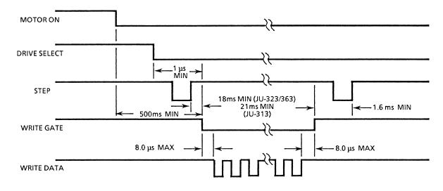
FIGURE 1-8 WRITE INITIATE TIMING
