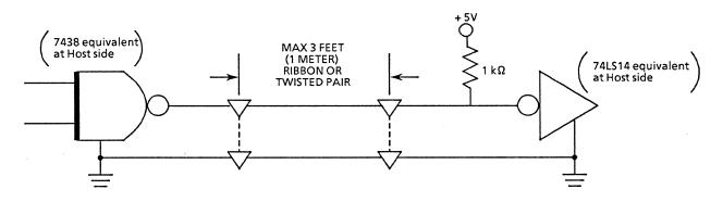
FIGURE 2-2 INTERFACE SIGNAL DRIVER/RECEIVER
