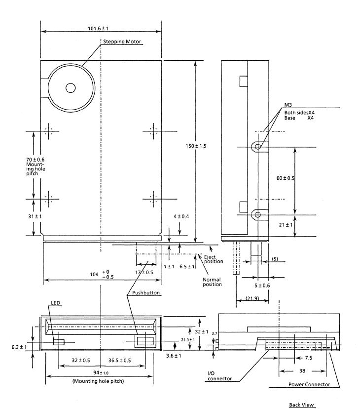
FIGURE 4-2. MECHANICAL DIMENSIONS
