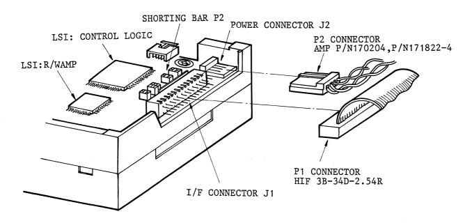
FIGURE 3-1 INTERFACE CONNECTORS LOCATIONS
