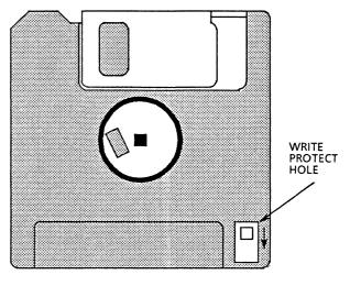
WRITE ENABLED HOLE CLOSED SLIDE MECHANICAL TAB AS SHOWN TO OPEN HOLE WRITE PROTECTED
