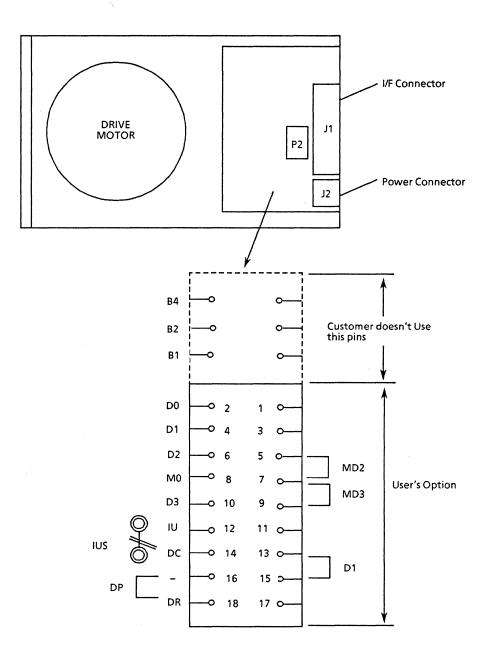
FIGURE 7-2 SHORTING BAR P2 PIN ASSIGNMENT
