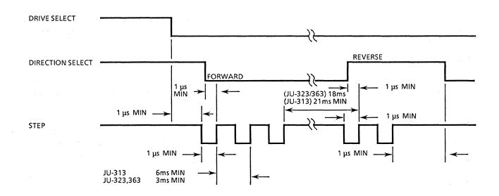
FIGURE 1-3 TRACK ACCESS TIMING
