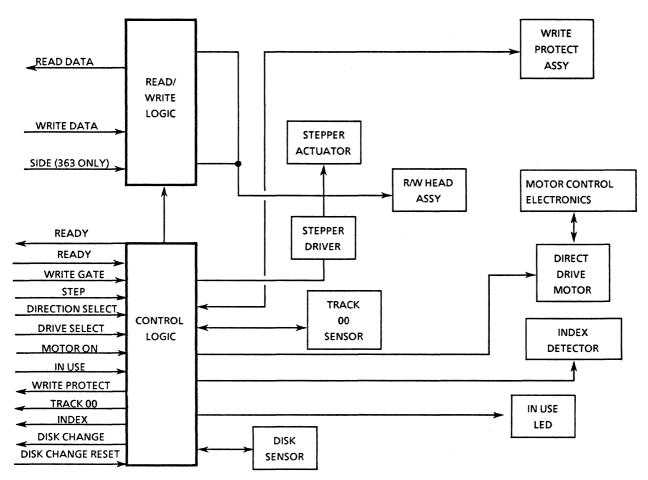
FIGURE 1-2 JU3X3 FUNCTIONAL DIAGRAM
