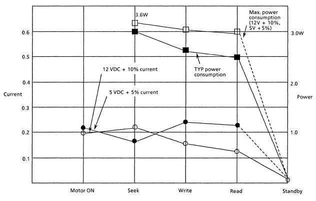
FIGURE 1-1 CALCULATION METHOD OF POWER CONSUMPTION
