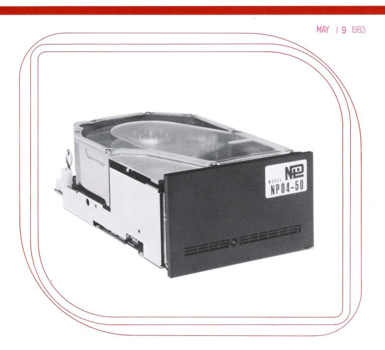
The NP04-50 disk drive is composed of 51/4-inch hard disk storage modules with a recording capacity of 50 megabytes on four fixed disks.
