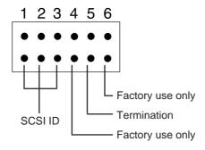
**Jumper locations 1, 2 and 3** are used to set the SCSI ID. Illustration shows how to install jumpers to set the SCSI ID.
