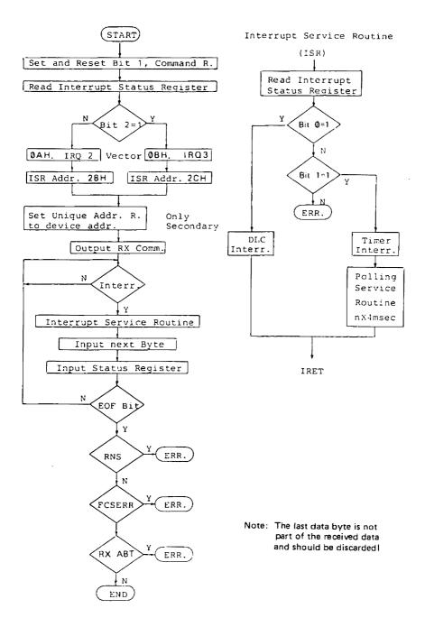
Figure 5.9 CPU Receive (2 of 2)
