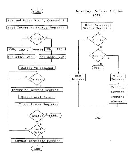
Figure 5.8 CPU Transmit (2 of 2)
