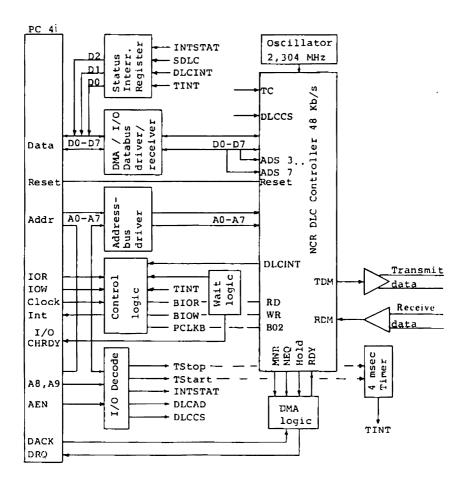
Figure 5.3 DLC Controller: Signal Flow
