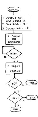
Figure 5.11 (1 of 2) DMA Receive
