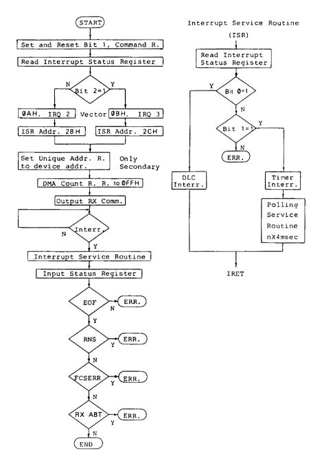
Figure 5.11 DMA Receive (2 of 2)
