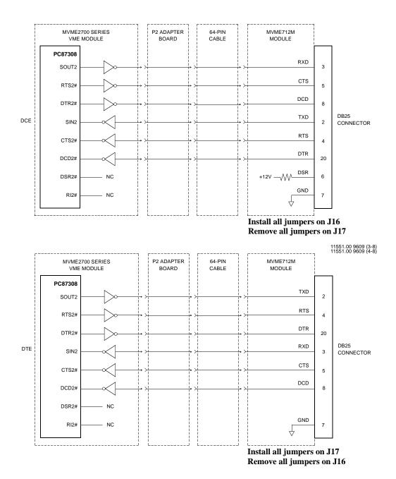
Figure 1-6. MVME712M Serial Port 2 DCE/DTE Configuration
