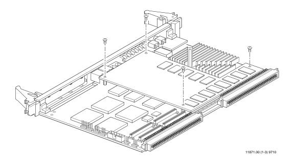
Figure 1-20. RAM200 Placement on MVME2700
