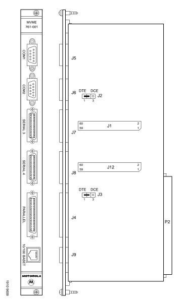
Figure 1-12. MVME761 Connector and Header Locations
