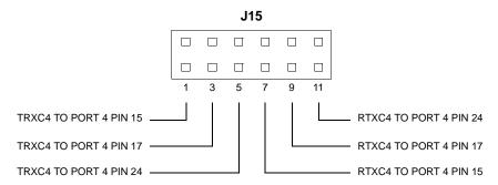
Figure 1-4. J15 Clock Line Configuration
