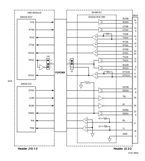
Figure 1-18. MVME761 EIA-530-DCE Configuration Port 3
