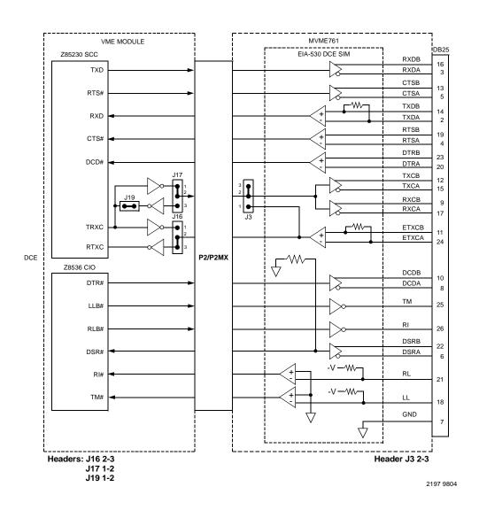
Figure 1-20. MVME761 EIA-530-DCE Configuration Port 4
