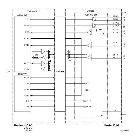
Figure 1-29. MVME761 X.21-DTE Configuration Port 4
