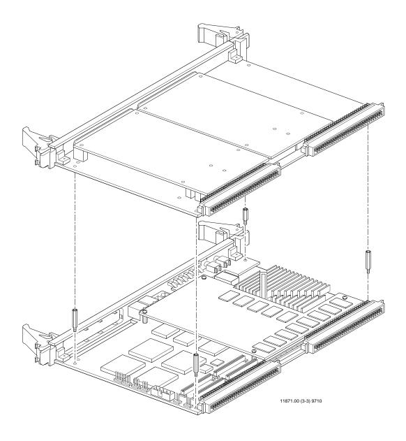
Figure 1-22. PMC Carrier Board Placement on MVME2700
