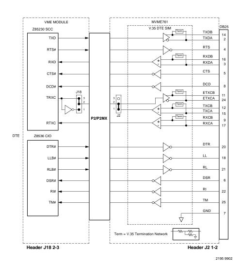
Figure 1-23. MVME761 V.35-DTE Configuration Port 3
