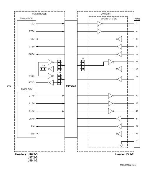
Figure 1-17. MVME761 EIA-232-D Port 4 DTE Configuration
