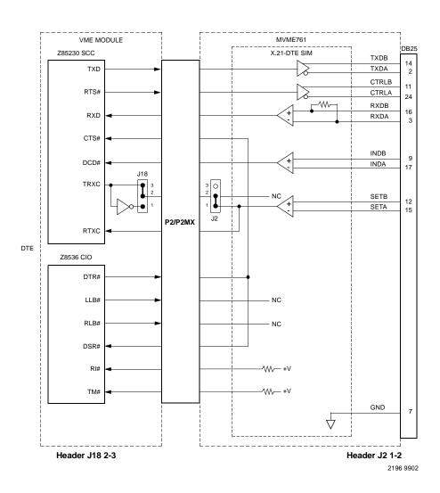
Figure 1-27. MVME761 X.21-DTE Configuration Port 3
