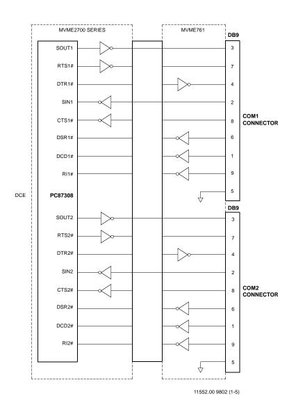
Figure 1-13. MVME761 Serial Ports 1 and 2 (DCE Only)
