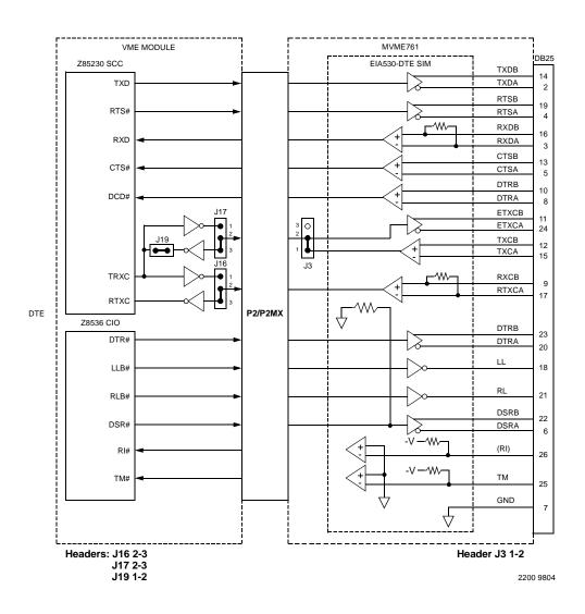
Figure 1-21. MVME761 EIA-530-DTE Port Configuration Port 4
