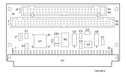
Figure 1-30. MVME761 Three-Row P2 Adapter
