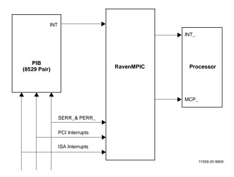
Figure 2-3. MVME2700 Interrupt Architecture
