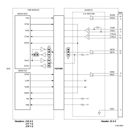
Figure 1-28. MVME761 X.21-DCE Configuration Port 4
