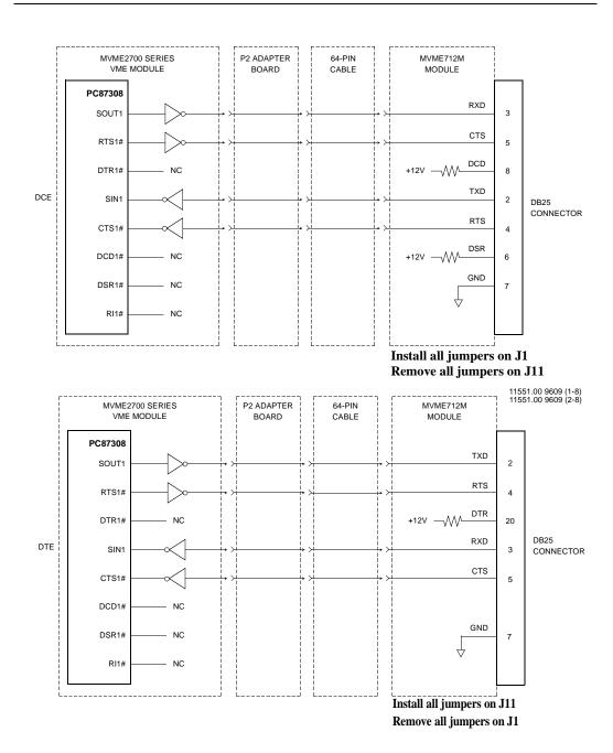
Figure 1-5. MVME712M Serial Port 1 DCE/DTE Configuration
