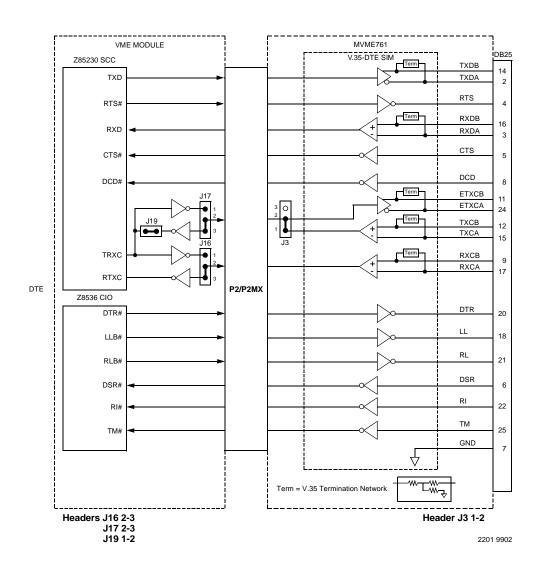
Figure 1-25. MVME761 V.35-DTE Configuration Port 4
