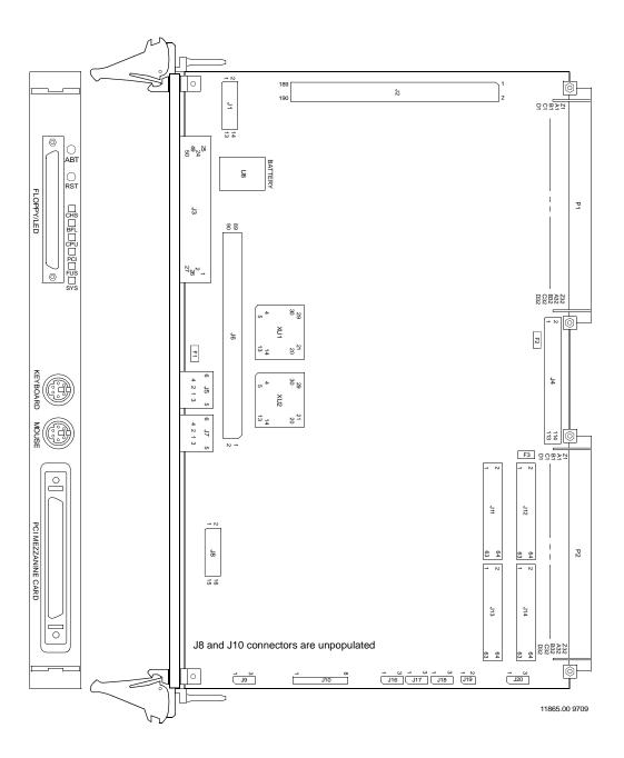
Figure 1-2. MVME2700 Switches, Headers, Connectors, Fuses, LEDs
