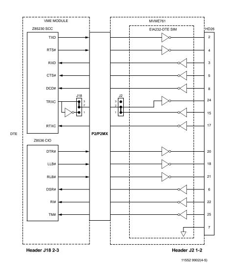
Figure 1-15. MVME761 EIA-232-D Port 3 DTE Configuration
