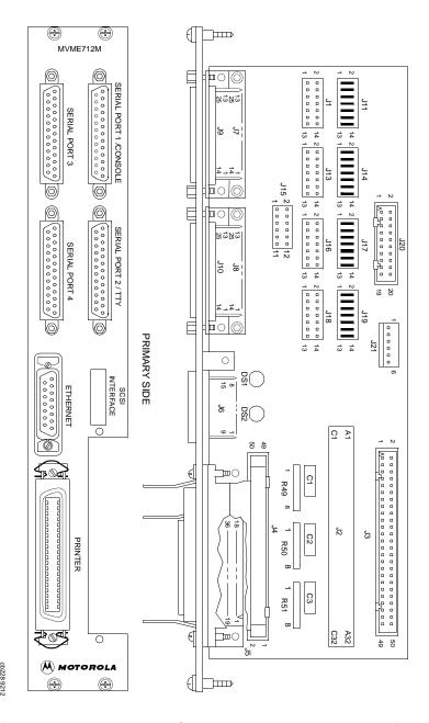
Figure 1-3. MVME712M Connector and Header Locations
