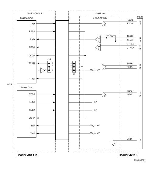
Figure 1-26. MVME761 X.21-DCE Configuration Port 3
