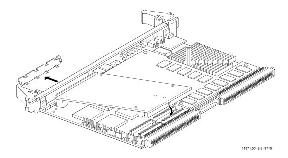
Figure 1-21. PMC Module Placement on MVME2700
