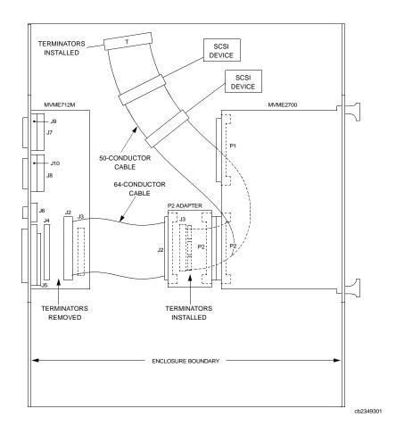
Figure 1-23. MVME712M/MVME2700 Cable Connections
