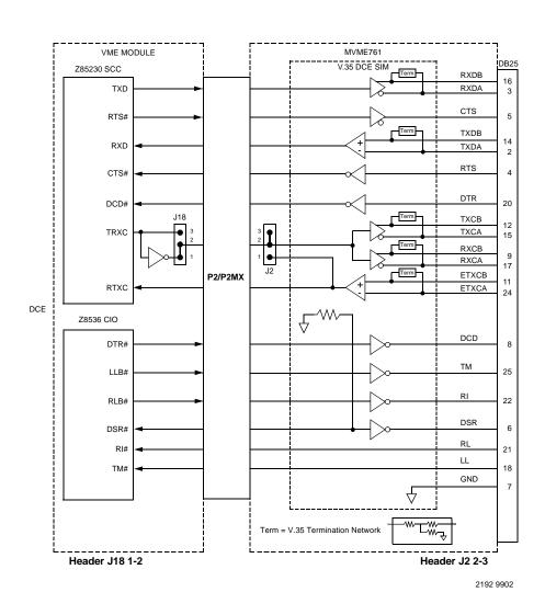
Figure 1-22. MVME761 V.35-DCE Configuration Port 3
