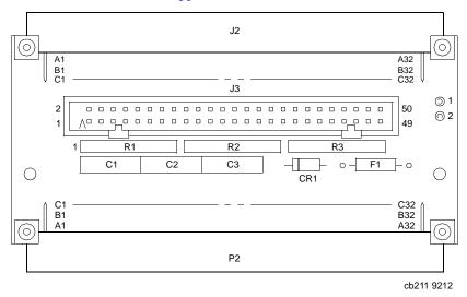
Figure 1-11. MVME712M Three-Row P2 Adapter
