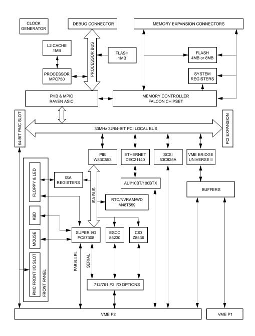
Figure 1-1. MVME2700 Base Board Block Diagram
