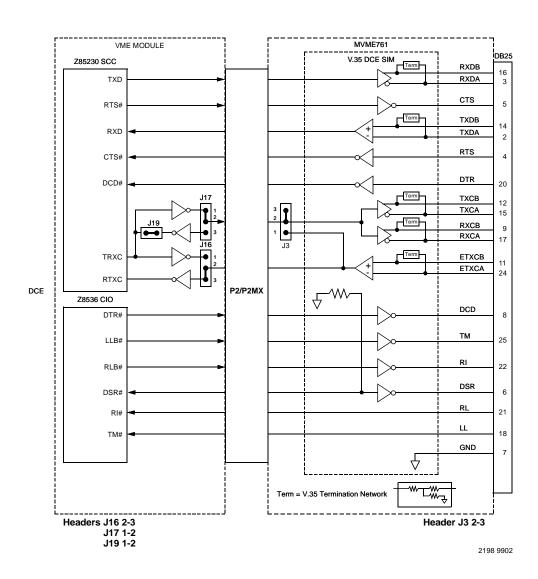
Figure 1-24. MVME761 V.35-DCE Configuration Port 4
