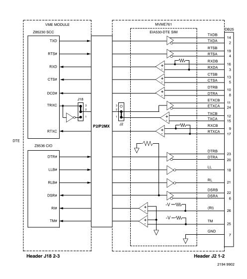
Figure 1-19. MVME761 EIA-530-DTE Configuration Port 3
