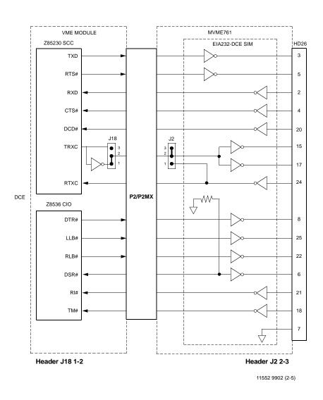
Figure 1-14. MVME761 EIA-232-D Port 3 DCE Configuration
