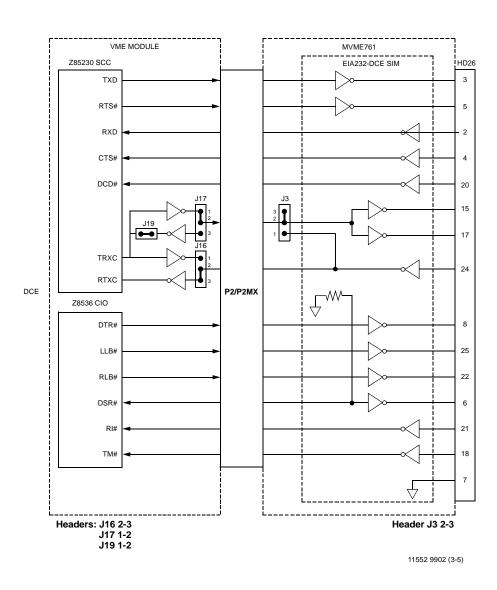
Figure 1-16. MVME761 EIA-232-D Port 4 DCE Configuration
