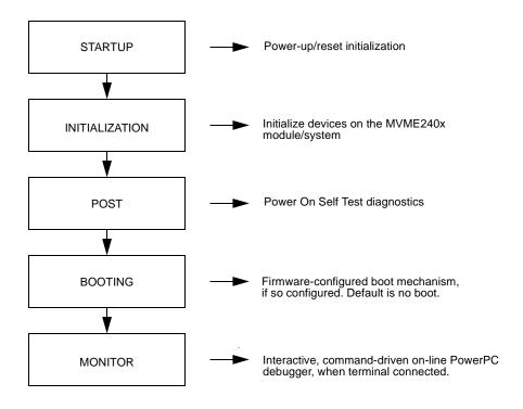
Figure 2-1. PPCBug Firmware System Startup
