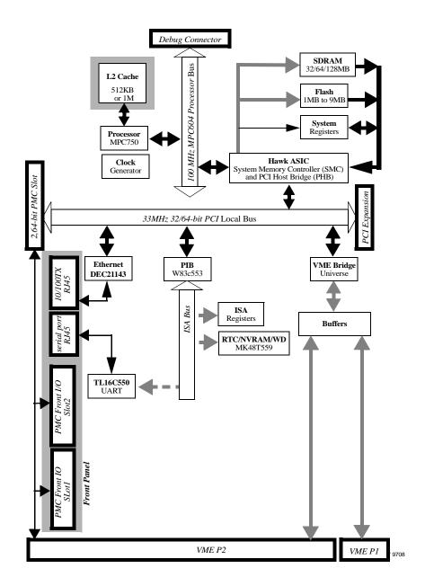
Figure 3-1. MVME240x Block Diagram
