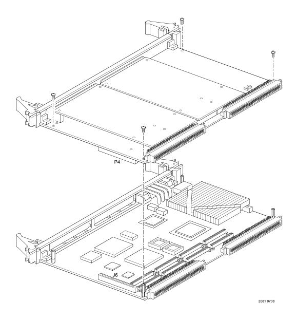
Figure 1-4. PMCspan-002 Installation on an MVME240x
