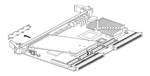
Figure 1-3. Typical Single-width PMC Module Placement on MVME240x
