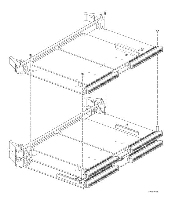
Figure 1-5. PMCspan-010 Installation on a PMCspan-002/MVME240x
