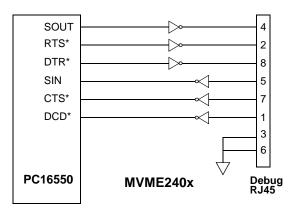
Figure 2-2. MVME240x DEBUG Port Configuration
