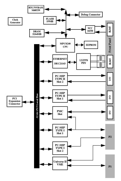
The following block diagram illustrates the architecture of the MVME2100 Single Board Computer.
