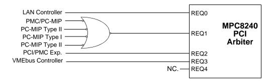
Figure 2-1. MVME 2100 PCI Arbitration
