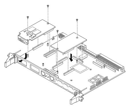
Figure 1-4. Typical Type II PC•MIP Placement on an MVME2100
