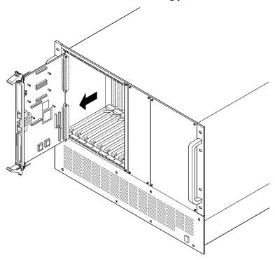
Figure 1-2. MVME2100 Installation and Removal From a VMEbus Chassis
