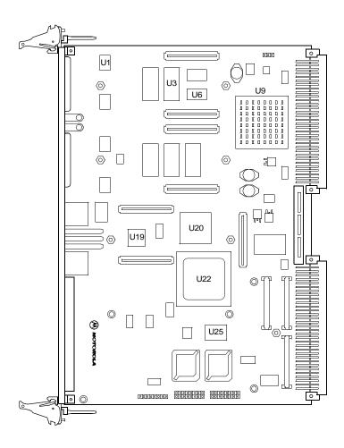
Figure B-1. Thermally Significant Components (Primary Side)
