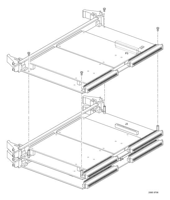
Figure 1-6. PMCspan-010 Installation on a PMCspan-001/MVME2100
