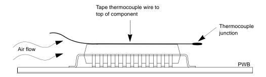
Figure B-4. Measuring Local Air Temperature
