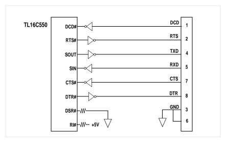
Figure 3-2. Asynchronous Serial Port Connections
