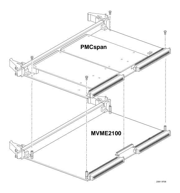
Figure 1-5. PMCspan-001 Installation on an MVME2100
