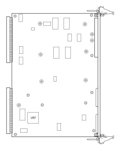
Figure B-2. Thermally Significant Components (Secondary Side)
