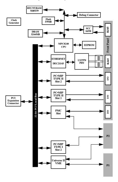
Figure 3-1. MVME2100 Block Diagram
