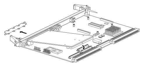
Figure 1-3. Typical Single-width PMC Module Placement on an MVME2100
