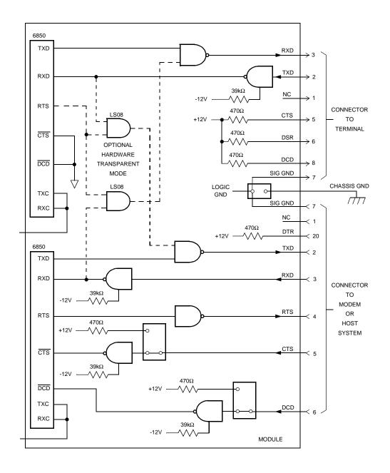
Figure A-1. Middle-of-the-Road EIA-232-D Configuration
