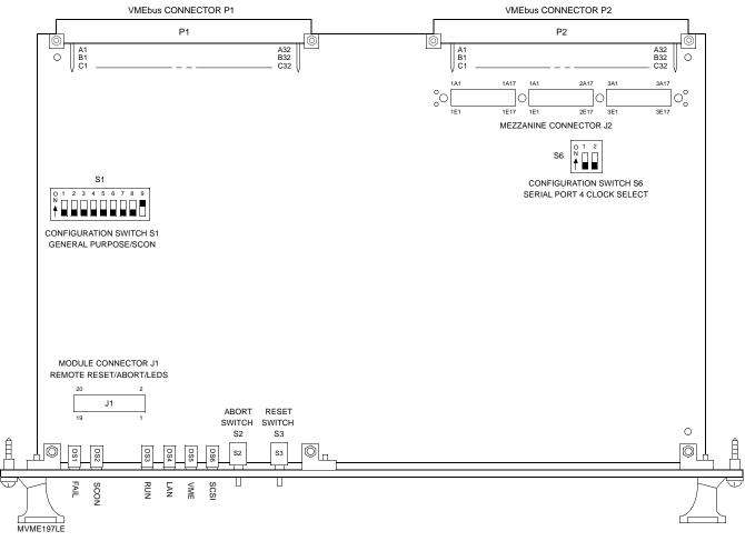
Figure 2-1. MVME197LE Switches, Connectors, and LED Indicators Location Diagram
