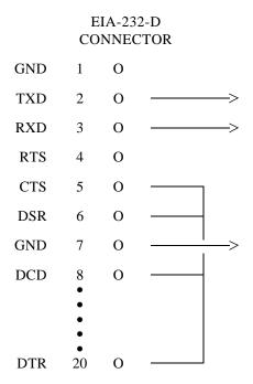
Figure A-2. Minimum EIA-232-D Connection
