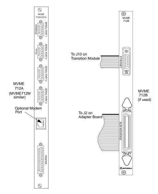
Figure 3-4. Typical Transition Module Peripheral Port Connectors
