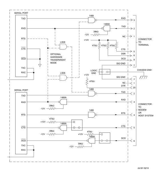
Figure E-1. Middle-of-the-Road EIA-232-D Configuration
