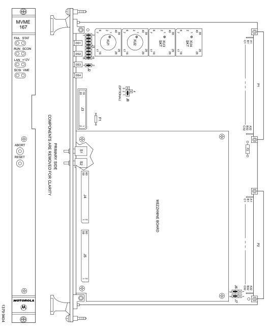
Figure 3-1. MVME167 Switches, Headers, Connectors, Fuses, and LEDs
