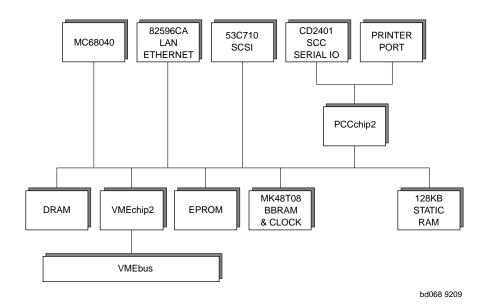
Figure 2-1. MVME167 General Block Diagram
