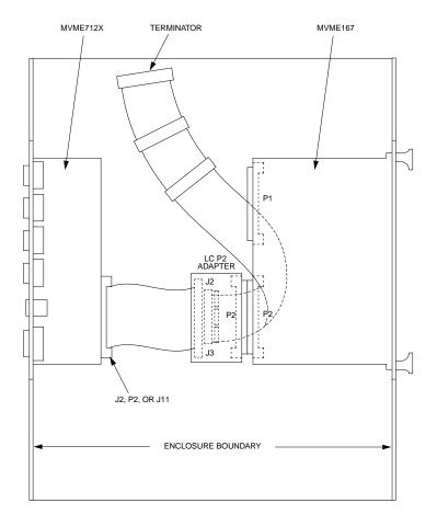
Figure 3-2. Typical Internal SCSI and Serial Port Connections
