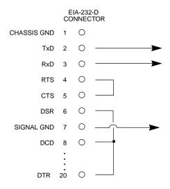
Figure E-2. Minimum EIA-232-D Connection
