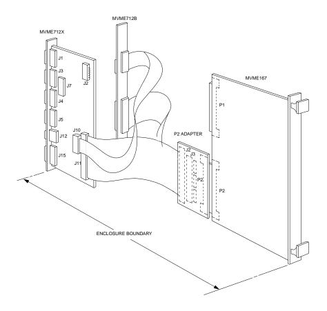
Figure 3-3. Using MVME712A/AM and MVME712B
