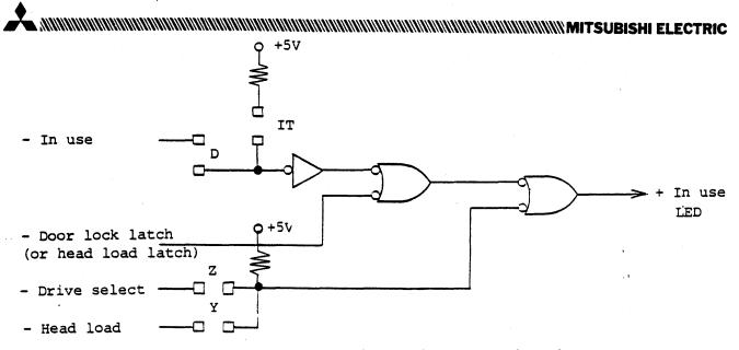
Fig. 6-4 In Use/Activity LED Circuit
