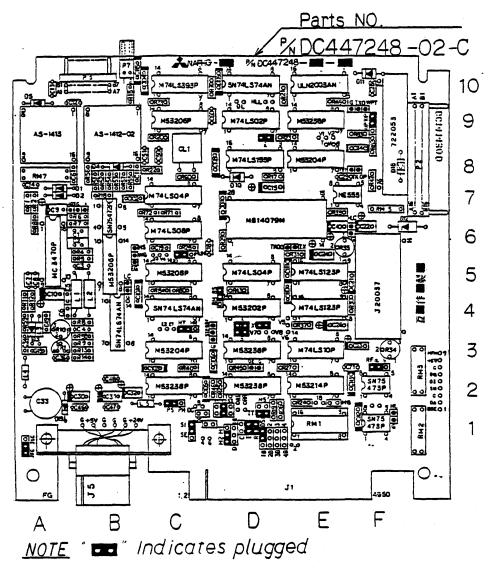
Fig. 6-1 Printed-Circuit Board Option Locations
