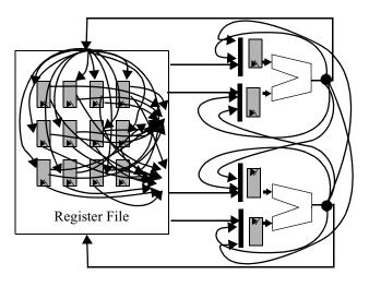
Figure 3: A pipelined processor with bypass links and multiple ALUs
