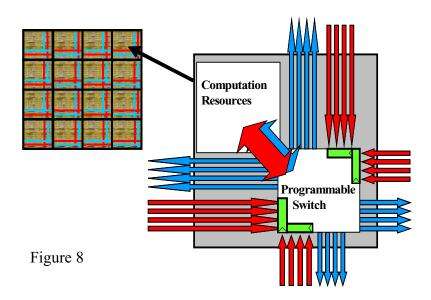
The static router is used to route the outputs of instructions on one tile to the inputs of the dependent instruc-
