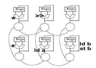
Figure 7: Mapping a dataflow graph on a generic distributed microprocessor containing 6 tiles.
