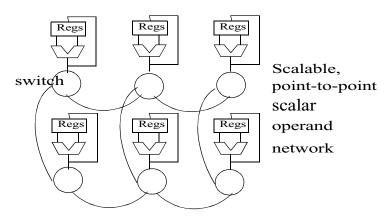
Figure 5: Scalar operand network based on a two dimensional, point-to-point routed interconnect
