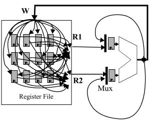
Figure 2: Scalar operand network in a pipelined processor with bypassing links added
