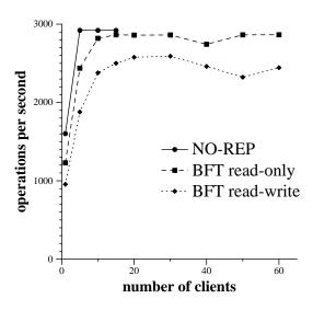
Figure 8-10: Throughput for operation 4/0 (with 4 KByte argument and 8 byte result).
