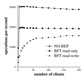
Figure 8-7: Throughput for operation 0/0 (with 8 byte argument and result).
