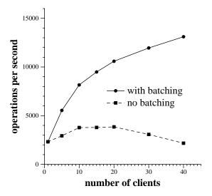
Figure 8-14: Throughput for operation 0/0 with and without request batching.
