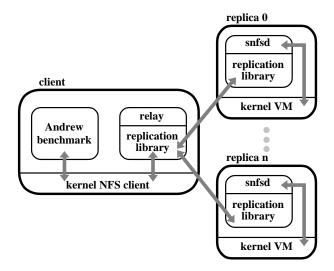
Figure 6-3: BFS: Replicated File System Architecture.
