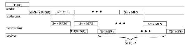
Figure 7-2: Performance model: time to send a message with l bytes that is fragmented. l' is the size of the message plus the number of bytes of protocol overhead ( $l' = RFS(l) + (NF(l) - 1) \times MFS$ ).
