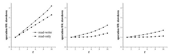
Figure 8-23: Predicted slowdown relative to the configuration with f=1 for increasing f and result size.
