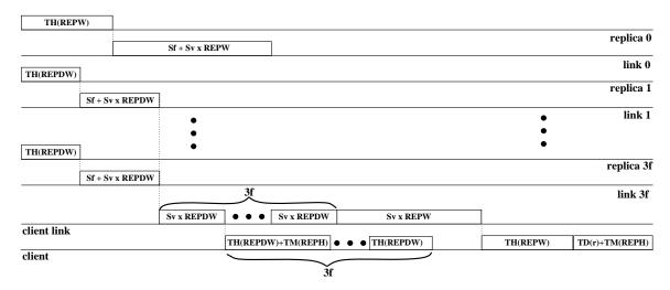
Figure 7-4: Communication time for replies that are not fragmented. *REPW* is the size of the reply frame with the result of the operation and *REPDW* is the size of a frame with a digest reply.
