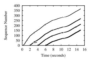
Figure 7: The CM scheduler apportions bandwidth well between simultaneous flows.
