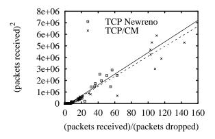
Figure 3: CM's rate control is TCP-friendly.
