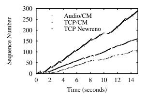
Figure 10: Performance of an adaptive audio application
