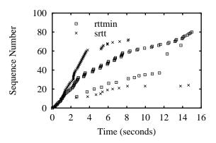
Figure 6: Sequence traces showing that exponential aging based on mean round-trip time is significantly inferior to using the minimum.
