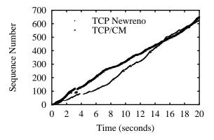
Figure 2: Sequence traces for TCP Newreno and TCP/CM, showing TCP/CM's true emulation of TCP
