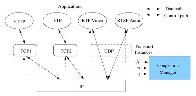
Figure 1: New sender architecture with centered around the Congestion Manager.
