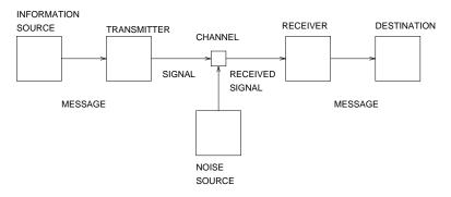
Figure 1-1: Shannon's schematic of a communication system.
