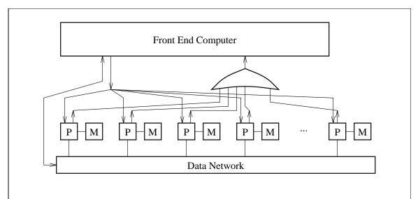
Figure 1-1: The organization of a SIMD computer. The front-end computer controls the processormemory pairs, through a broadcast network, on a clock-cycle by clock-cycle basis. The 'or' network accepts a bit from each processor and delivers the logical 'or' of all the bits to the front-end. The front-end also controls the data network.
