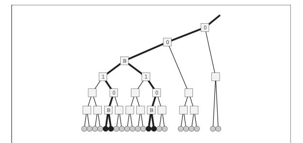
Figure 2-6: Steering a token down the diagnostic network. The address is decoded digit-serially, where each digit is 0, 1, or B, representing a selection of the left subtree, right subtree, or both subtrees, respectively. The example shows the selection made by the address 00B10B.
