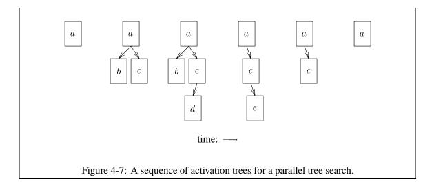
In a parallel implementation, however, calls to b and c may run concurrently, and the last-infirst-out discipline for allocating activation frames does not work. A parallel implementation must use a *tree* of activation frames rather than a *stack* of activation frames.<sup>5</sup>
