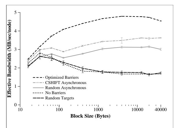
Figure 3-6: The effect of interleaving. The two asynchronous block transfer versions use packet interleaving to achieve about twice as much bandwidth as the corresponding normal block transfers. The version with barriers still performs much better, but it applies only when the communication can be structured as a sequence of permutations. The asynchronous block-transfer interface avoids this requirement.
