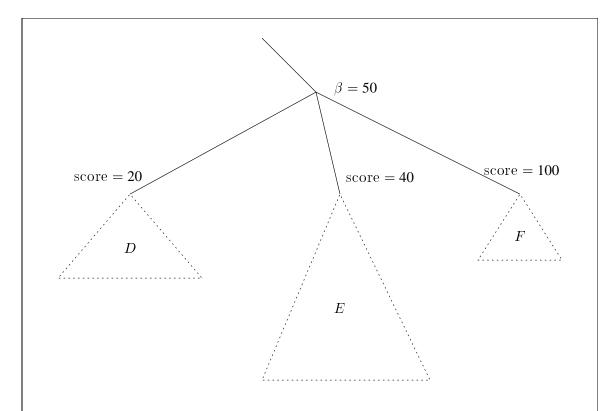
Figure 5-6: Jamboree search sometimes does less work than a serial algorithm. The value of  $\beta$  is 50. The first child, D is searched and the score is determined to be 20. The second child, E, is a large subtree with a score of 40. Jamboree search might search the third child, F, which has a score of at least 100, before E has been finished, and Jamboree might abort the expensive search of E.
