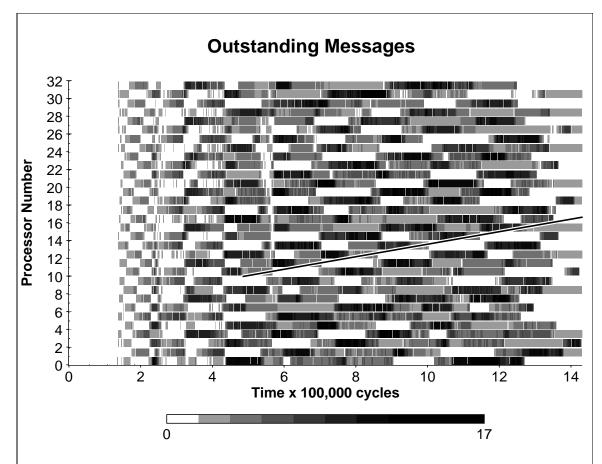
Figure 3-4: The total number of packets in the network headed to any given processor at any given time. Time is measured in 33-megahertz clock cycles. The diagonal line superimposed on the drawing follows the pattern of systematic interference caused by target collisions.
