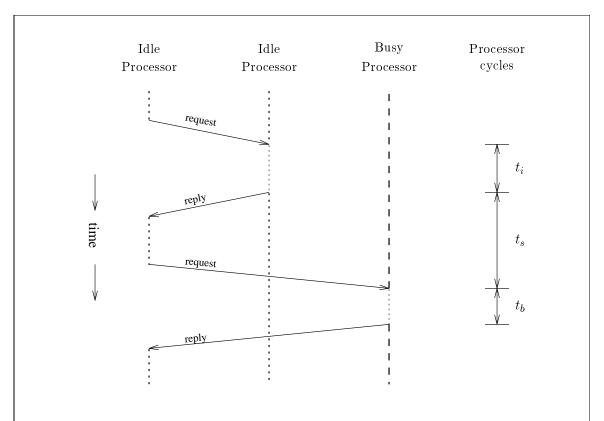
Figure 5-19: The relationship of  $t_b$ ,  $t_i$  and  $t_s$  in the SWAMP program. The time required of a busy processor to service a request is  $t_b$ . The time for an idle processor to service a request is  $t_i$ . The round trip time from when a denial is sent by a processor to back to an idle requesting processor, to the time that the requestor's next request arrives at a processor is  $t_s$ .
