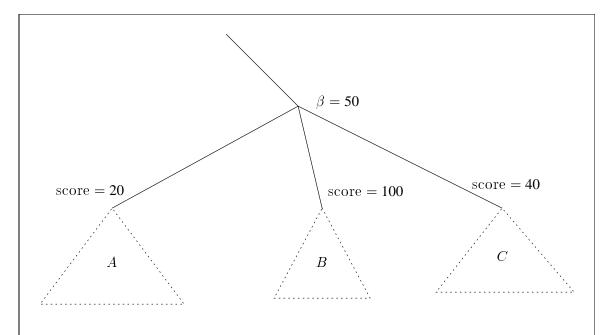
Figure 5-5: Jamboree search sometimes does more work than a serial algorithm. In this case the value of  $\beta$  is 50, so as soon as a child is found with score  $\geq$  50, a serial algorithm would stop examining children. Jamboree search, like a serial algorithm, searches the first child, A, obtaining a value of 20. Then Jamboree searches B and C in parallel, aborting the search of C only when the value of B is determined. A serial algorithm would never search C.
