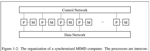
nected by two networks: a data network and a control network.
