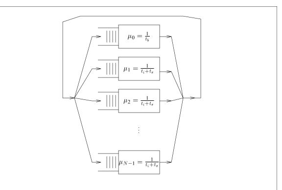
Figure 5-22: This Jackson network models the swamping problem. The critical parameter is the *leverage*  $z = t_b/(t_s + t_i)$ .
