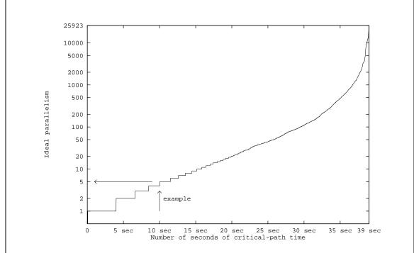
Figure 5-14: The sorted ideal-parallelism profile shows how the ideal parallelism is distributed. For example, (shown with arrows) for 10 seconds there is less than five-fold parallelism.
