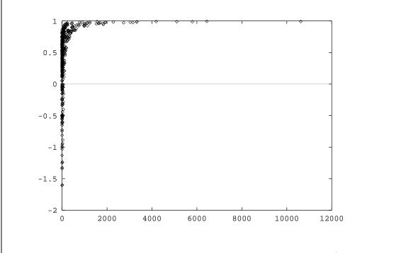
Figure 5-17: Plot of the relative residuals of 3.682 + 3.978C as a function of W/P. The residuals are clearly an increasing function of W/P.
