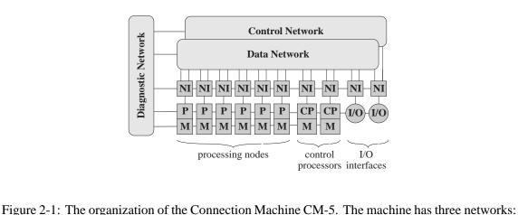
Figure 2-1: The organization of the Connection Machine CM-5. The machine has three networks: a data network, a control network, and a diagnostic network. The data and control networks are connected to processing nodes, control processors, and I/O channels via a network interface.
