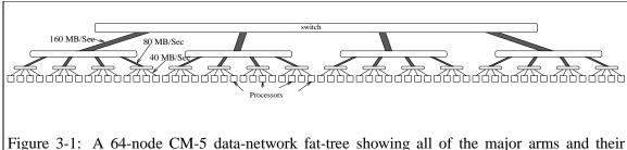
Figure 3-1: A 64-node CM-5 data-network fat-tree showing all of the major arms and their bandwidths (in each direction). One needs to cut only a single major arm to find the worst bisection for a given message pattern.
