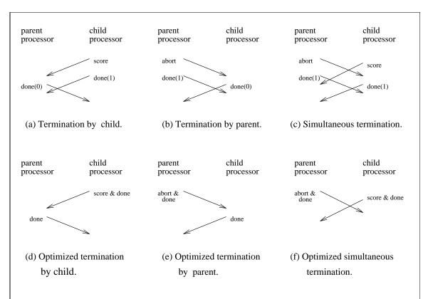
Figure 4-8: Three possible ways to for a frame to terminate (left to right). In the naive implementation (top), either a 'score' message or an 'abort' message can trigger the 'done' messages, which contain a message-count. In the optimized implementation (bottom), the 'done' message is piggybacked with the 'score' or the 'abort' message.
