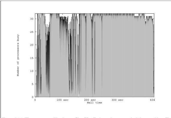
Figure 5-15: The processor utilization profile of StarTech running on a typical chess position. The horizontal axis is the wall time, and the height of the curve is the number of busy processors. The shaded area under the curve represents processor-cycles spent on useful work.
