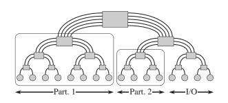
Figure 2-2: A binary fat-tree. Processors are located at the leaves, and the internal nodes are switches. Unlike an ordinary binary tree, the channel capacities of a fat-tree increase as we ascend from leaves to root. The hierarchical nature of a fat-tree can be exploited to give each user partition a dedicated subnetwork which cannot be interfered with by any other partition's message traffic. The CM-5 data network uses a 4-ary tree instead of a binary tree.
