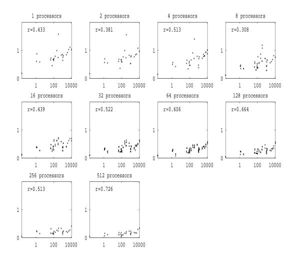
Figure 5-12: A scatter plot of the serial run time against the work efficiency. The horizontal axis of each scatter plot is the serial run time in seconds. The vertical axis is the work efficiency (the ratio of the serial run time to the parallel work.) The scales of both axes are the same for each scatter plot. One scatter plot is shown for each machine size. The sample correlation coefficient (r) is shown in the upper left hand corner of each scatter plot.
