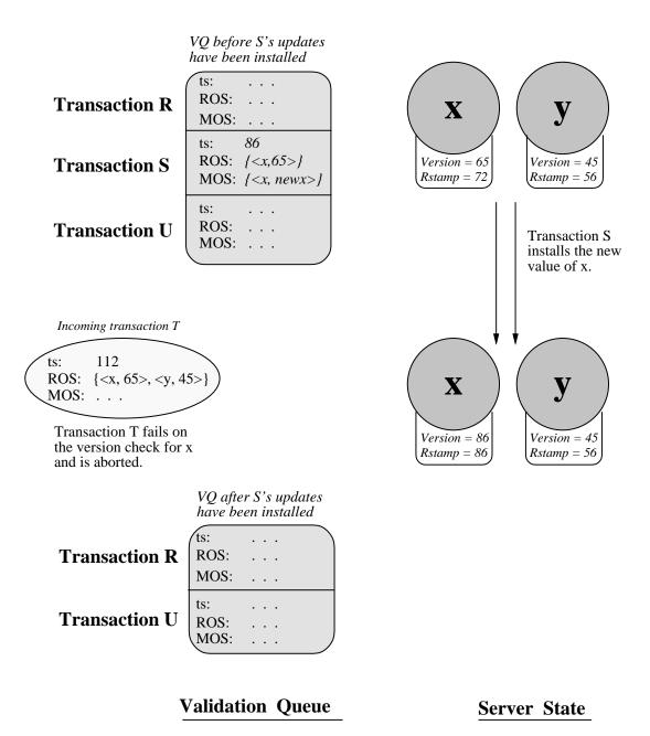
Figure 3-4: Validation failure on the version check
