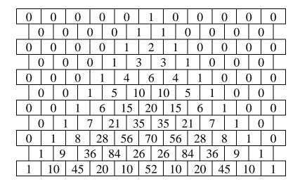
Figure 2-4: A spacetime diagram showing the cells of a one-dimensional CA that generates Pascal's triangle. The automaton starts out with a single 1 in a background of 0's, and thereafter, each cell is the sum (mod 100) of the two cells above it. The last two rows show the effect of truncating the high digits.
