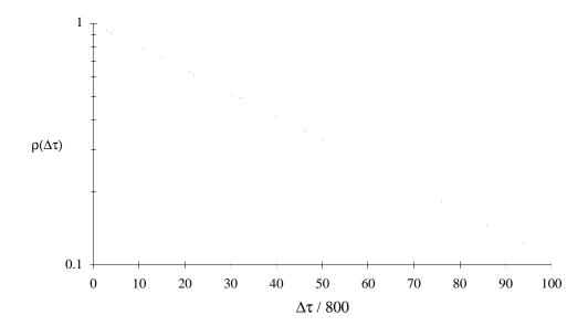
Figure 5-12: A semilogarithmic plot of the time autocorrelation function of the radius of gyration for the polymer with N=140. The dotted line is chosen to have the same area under the curve, and its slope gives a measure of the relaxation time.
