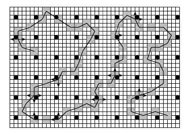
Figure 5-9: Realization of the polymer strand in the bond fluctuation method with N=60. All monomers containing a dot can move in parallel without interference, and the arrows show all moves allowed by the constraints.
