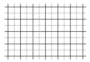
Figure 3-4: The Margolus neighborhood: the entire array is partitioned into  $2\times2$  blocks, and the new state of each block only depends on the four cells in that block. The blocking can be changed from even to odd (solid to dotted) between time steps in order to couple all the blocks.
