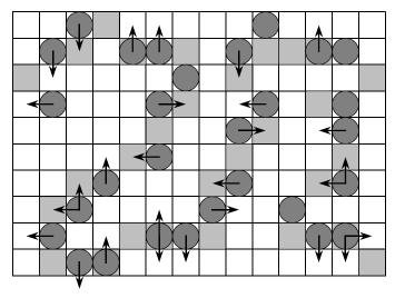
Figure 5-6: Abstract CA representation of the continuous polymer strand using the double space algorithm with N=58. The odd monomers, indicated by circles, are currently selected to move, and the arrows show all possible moves. The comparatively large number of available moves makes the polymer very flexible.
