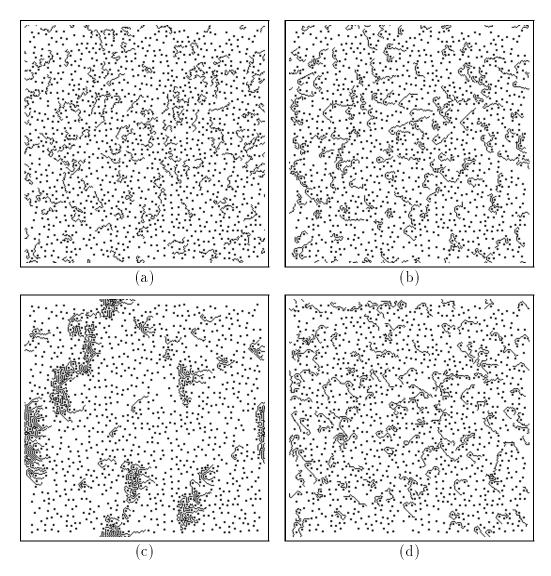
Figure 5-15: Electrophoresis demonstration on CAM-6. (a) Initial equilibrium configuration consisting of 128 polymers with N=30 in a background of 1000 immovable  $2\times 2$  blocks. (b) After 100 cycles of the rule, most of the polymers have become caught on an obstruction. (c) After 100,000 cycles of the rule, the polymers have drifted around the space until most are caught in one of a few clumps. (d) A configuration showing the effect of switching the direction of the field.
