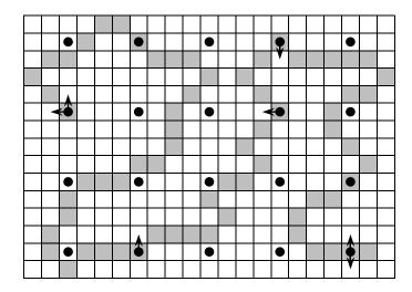
Figure 5-4: Another CA representation of the polymer having either nearest or next nearest neighbor connections. The lattice is finer than in the previous model while N=68 is comparable. Dots indicate active cells, and the arrows show all possible moves.
