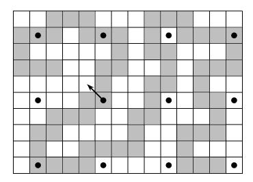
Figure 5-3: A simple CA realization of the polymer strand using a lattice model having only nearest-neighbor connections. Here, N = 65. Dots mark the cells from which monomers may move in parallel. The arrow indicates the only possible move.
