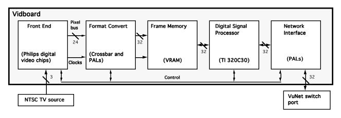
Figure 3: Block diagram of the Vidboard
