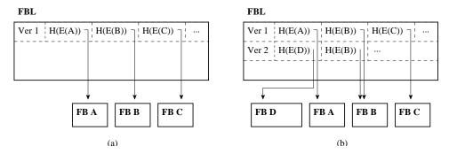
Figure 1: File Block List and File Blocks: (a) shows a file with three equal sized blocks, (b) shows how a new version can be added by updating the file block list and adding a single new file block.
