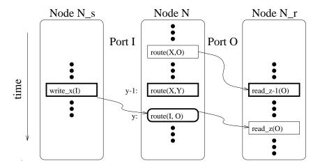
Figure 9: **Dependent instructions of a communication instruction.** Each long rectangle represents an execution node, and each wide rectangle represents an instruction. Spaces between execution nodes are ports. Edges represent flow of data. The focal instruction is the thick rounded rectangle. Its dependent instructions are in thick regular rectangles.
