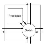
Figure 3: Communication ports for the static network on a prototype tile. Each switch on a tile is connected to its processor and its four neighbors via an input port and an output port. The figure is not drawn to scale.
