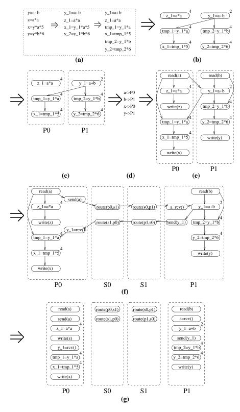
Figure 6: An example of the program transformations performed by RAWCC . (a) shows the initial program undergoing transformations made by *initial code transformation*; (b) shows result of *task graph builder*; (c) shows result of *instruction partitioner*; (d) shows result of *data partitioner*; (e) shows result of *basic block stitcher*; (f) shows result of *communication code generator*; (g) shows final result from *event scheduler*.
