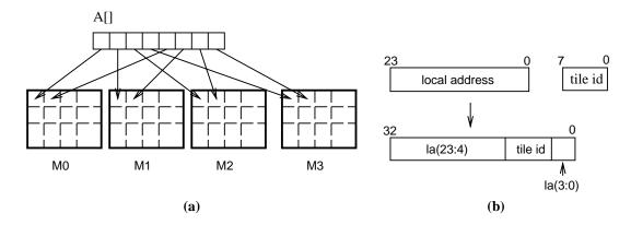
Figure 7: Low order interleaving. (a) An array object is interleaved element-wise across four memories. (b) A 24 bit local address combines with with an 8 bit tile id to form an address to a low-order interleaved memory. The interleaving granularity determines the point at which the symbolic address is split.  $(sizeo f(low\_order\_chunk) = log_2(16))$
