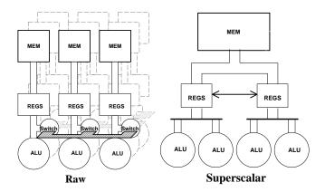
Figure 2: Internal organization of Raw processors versus superscalars. The Raw microprocessor distributes the register file and communicates between ALUs on a software-exposed, point-to-point interconnect. In contrast, a superscalar contains clusters of a register file and several function units, and it communicates between these components via busses hidden from the software.
