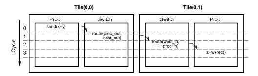
Figure 4: The end-to-end latency of a single-word message between neighbors is four cycles. In this example, both the send and the receive are performing useful computation, so that the effective overhead is only two cycles.
