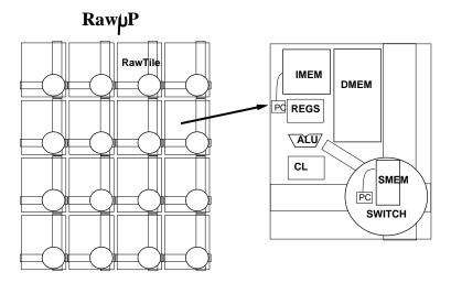
Figure 1: Raw $\mu$ P composition. A typical Raw system might include a Raw microprocessor coupled with off-chip RDRAM and stream-IO devices.
