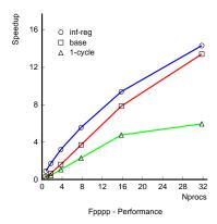
Figure 8: **Performance of fpppp-kernel under various machine configurations.** *Base* is the baseline machine; *inf-reg* is a machine with infinite number of registers per tile; *1-cycle* is a machine with single-cycle instructions. The cycle count for baseline number of *base* and *inf-reg* is 7478, and the cycle count of the baseline number of *1-cycle* is 3998.
