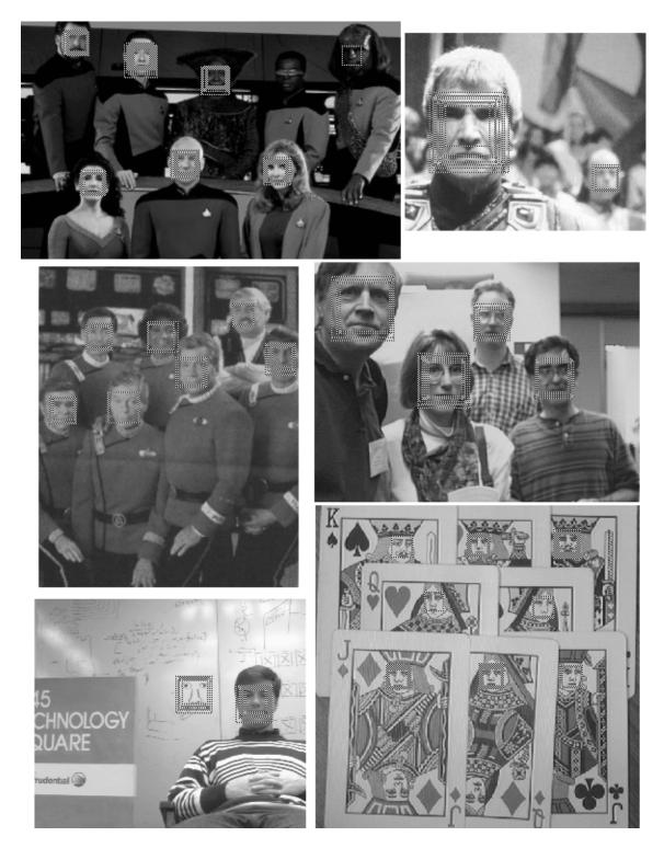
Figure 2-16: Some face detection results by our system. The upper and middle left images show that the system finds faces in complex scenes without making many false detects. The upper and middle right images show the system working successfully across different scales. The lower two images show that the same system detects real faces and face drawings equally well.
