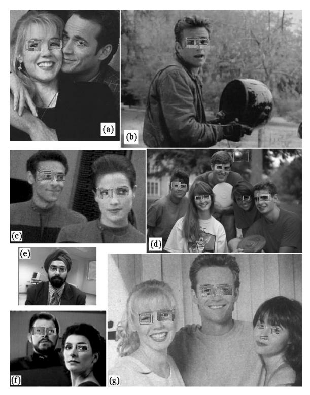
Figure 3-8: (a): The system misses Dylan's partly occluded right eye. (d): The system makes one false detect and misses the right eye of the two people on the right. (f): Misses Deanna Troi's right eye. (g): Brenda's nostril is mistaken for an eye. Notice that the system still detects Brenda's eyes successfully even though her head is significantly tilted.
