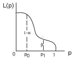
Figure 6-2: A typical operating characteristic function of the sequential ratio test
