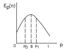
Figure 6-3: The typical shape of the average sample number of the sequential ratio test
