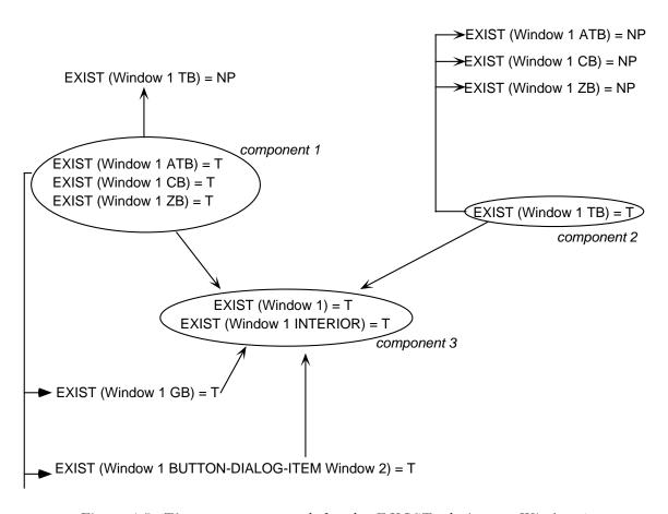
Figure 4-5: The component graph for the EXIST relation on Window 1
