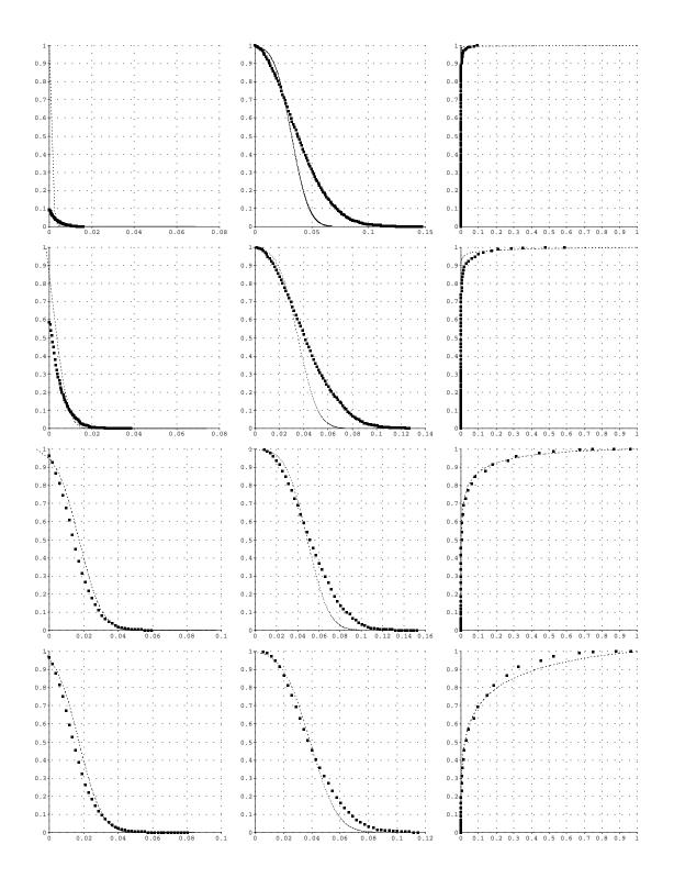
**Figure 4-2:** Comparison of predicted to empirical curves for probability of false alarm, probability of detection, ROC curves. The empirical curves are indicated by boxes. The axes for graphs, from left to right, are  $(x, y) = (\theta, P_F), (\theta, P_D)$ , and  $(P_F, P_D)$ . For all graphs,  $m = 10, \sigma_0 = 2.5$ . From top to bottom, n = 10, 100, 500, 500, occlusion = 0, 0, 0, 0.25.
