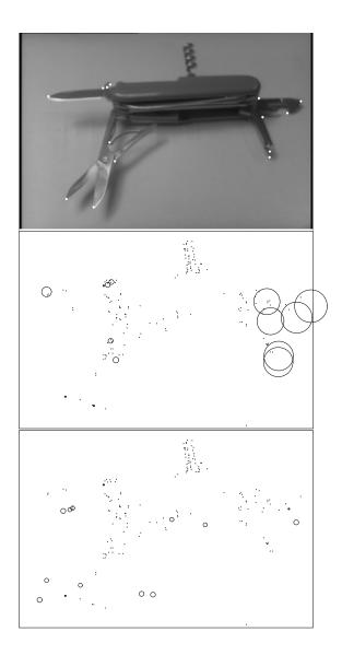
Figure 6-13: The top figure shows the original image, with the feature points chosen for the model indicated in white. The middle figure is a correct hypothesis that exceeded the predicted threshold, and the bottom shows an incorrect one.
