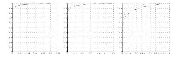
**Figure 5-4:** Comparison of empirical ROC curves for Schemes 1 and 3. In all graphs the ROC curve for Scheme 1 is above that of Scheme 3. The axes are  $(x, y) = (P_F, P_D)$ . For all graphs, m = 10, occlusion = 0,  $\sigma_0 = 2.5$ . From left to right, n = 10, 100, 500.
