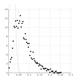
Figure 6-8: The histogram for the weights of incorrect hypotheses chosen from the original image. Note that the mean and variance greatly exceeds those of the predicted density of  $W_{\overline{H}}$  for m = 30, n = 248.
