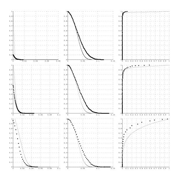
**Figure 5-3:** Comparison of predicted to empirical curves for probability of false alarm, probability of detection, and ROC curves for Scheme 3. The empirical points are indicated by boxes. The axes for graphs, from left to right, are  $(x, y) = (\theta, P_F), (\theta, P_D)$ , and  $(P_F, P_D)$ . For all graphs, m = 10, occlusion = 0,  $\sigma_0 = 2.5$ . From top to bottom, n = 10, 100, 500.
