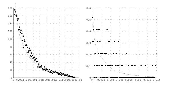
**Figure 3-5:** Distributions  $f_{V_M}(v)$  and  $f_{V_M}(v \mid m = 1)$  for v > 0. For these distributions,  $\sigma_0 = 2.5$ . Note that the scale of the y axis in the first graph is approximately ten times greater than that of the second.
