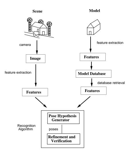
Figure 1-1: Stages in model based recognition.
