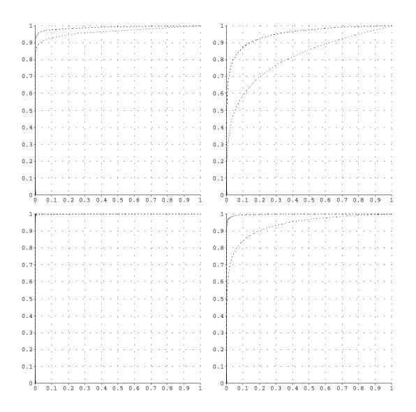
**Figure 5-2:** The graphs show the comparison of ROC curves for Scheme 1 (top curve) versus Scheme 3 (bottom curve). The x and y axes are  $P_F$  and  $P_D$ , respectively. Increasing  $(P_F, P_D)$  corresponds to a decreasing threshold for the direction of The (m,n) pairs are (10,100), (10,500), (30,100), and (30,500). For all graphs, occlusion = 0 and  $\sigma_0 = 2.5$ .
