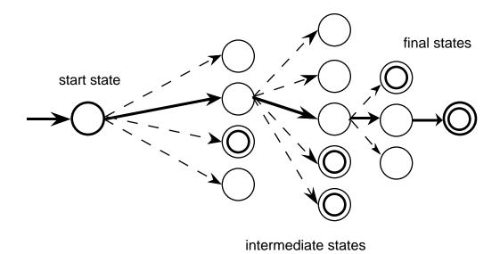
Figure 2.1: Using ordered depth-first search to choose a path in state space.
