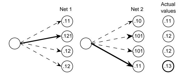
**Figure 3.1**: Network 1 predicts values that are very close to the actual values while network 2 has a sum of square error that is more than twelve times as large; however, because network 2 has done a better job of *ordering* the states, it choose the best state.
