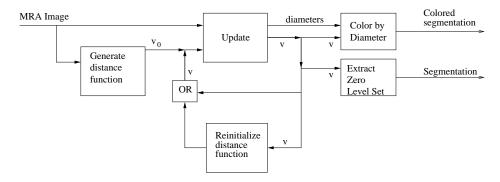
Fig. 6. Overview of segmentation algorithm.
