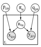
Figure 1: Graphical model representation for the symmetric parameterization of the Separable Mixture Model (SMM).
