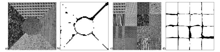
Figure 13: (a), (c) Two mixture images containing 5 textures each. (b), (d) The image segmentation obtained based on the ACM.
