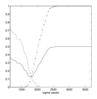
Figure 15: The effect of the basis function width ( $\sigma$ ) on the performance of an RBF module. Left: RBF-module miss rate (dashed line), false-alarm rate (dotted line) and their mean (solid line), plotted against  $\sigma$ . The values of  $\sigma$  shown on the abscissa range from half the minimal distance up to the maximal distance among RBF-module "centers" (training views) in the input space.
