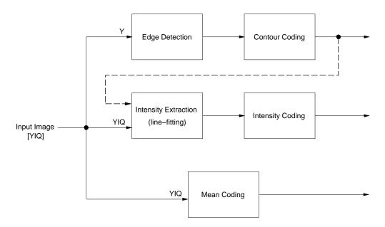
Figure 4: Block Diagram of Encoder
