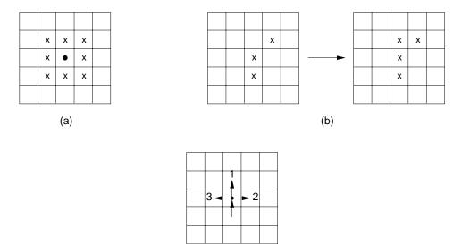
Figure 2: (a) An 8-connected edge map; (b) 8-connected to 4-connected transformation; (c) Possible directionals for a 4-connected map.
