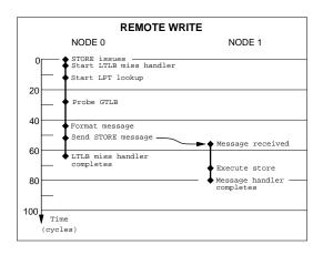
Figure 9: Timeline for remote read and write accesses.
