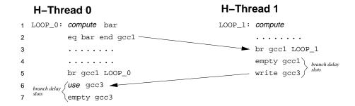
Figure 6: Loop synchronization between two H-Threads using MAP global CC registers.
