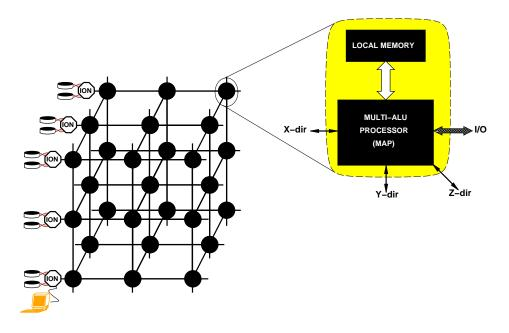
Figure 1: The M-Machine architecture.
