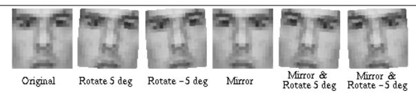
Figure 11: Artificially generating *virtual examples* of face patterns. For each original face pattern in our training database, we can generate a few new face patterns using some simple image transformations. We artificially enlarge our face database in this fashion to obtain a more comprehensive sample of face patterns.
