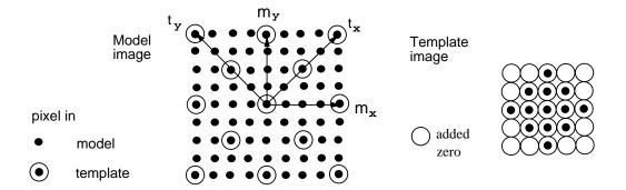
Figure 1: A  $5 \times 5$  template image is obtained from a  $9 \times 9$  model image using parameters  $s_x = s_y = 2$  and  $\tau = 45$  degrees.
