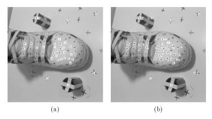
Figure 8: Re-projection onto the tenth frame. Epipoles are computed via fundamental matrix (see text) using the implementation of [21]. (a) Large base situation (structure computed between first and fifth frames): average error 1.62 with std of 1.2. (b) Small base-line situation (structure computed between first and second frames): average error 13.87 with std of 9.47.
