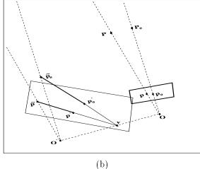
Figure 3: (a) Relative affine Structure:  $k = \frac{z_o}{z} \frac{d_p}{d_o}$ . (b) Affine structure under perspective (when  $\pi$  is at infinity). Note that the rays  $\overline{OP}$  and  $\overline{O'\tilde{p}}$  are parallel, thus the homography is the rotational component of motion.
